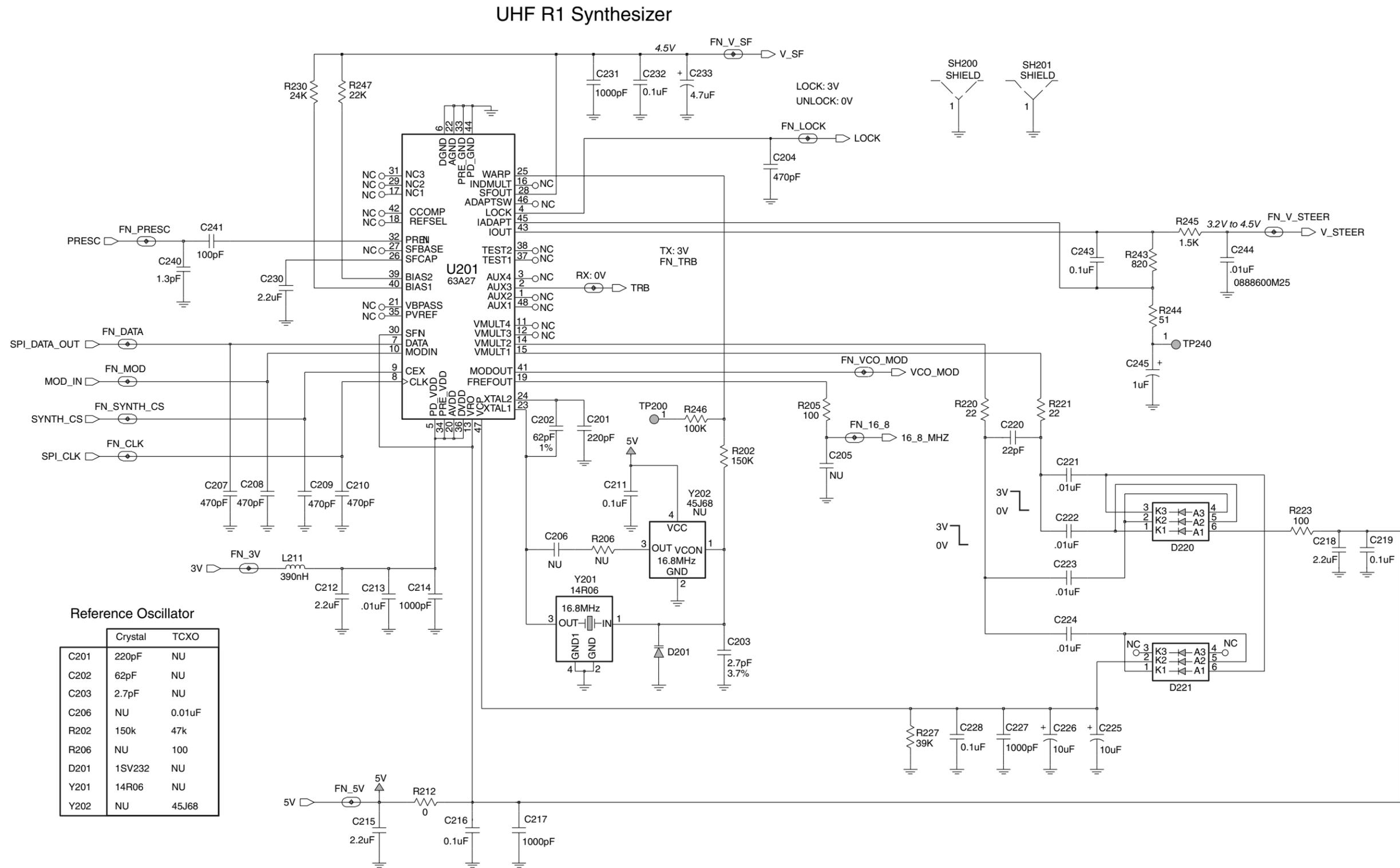
Figure 12-6. UHF (403-440 MHz) Synthesizer Schematic Diagram (8486635Z03-O)
