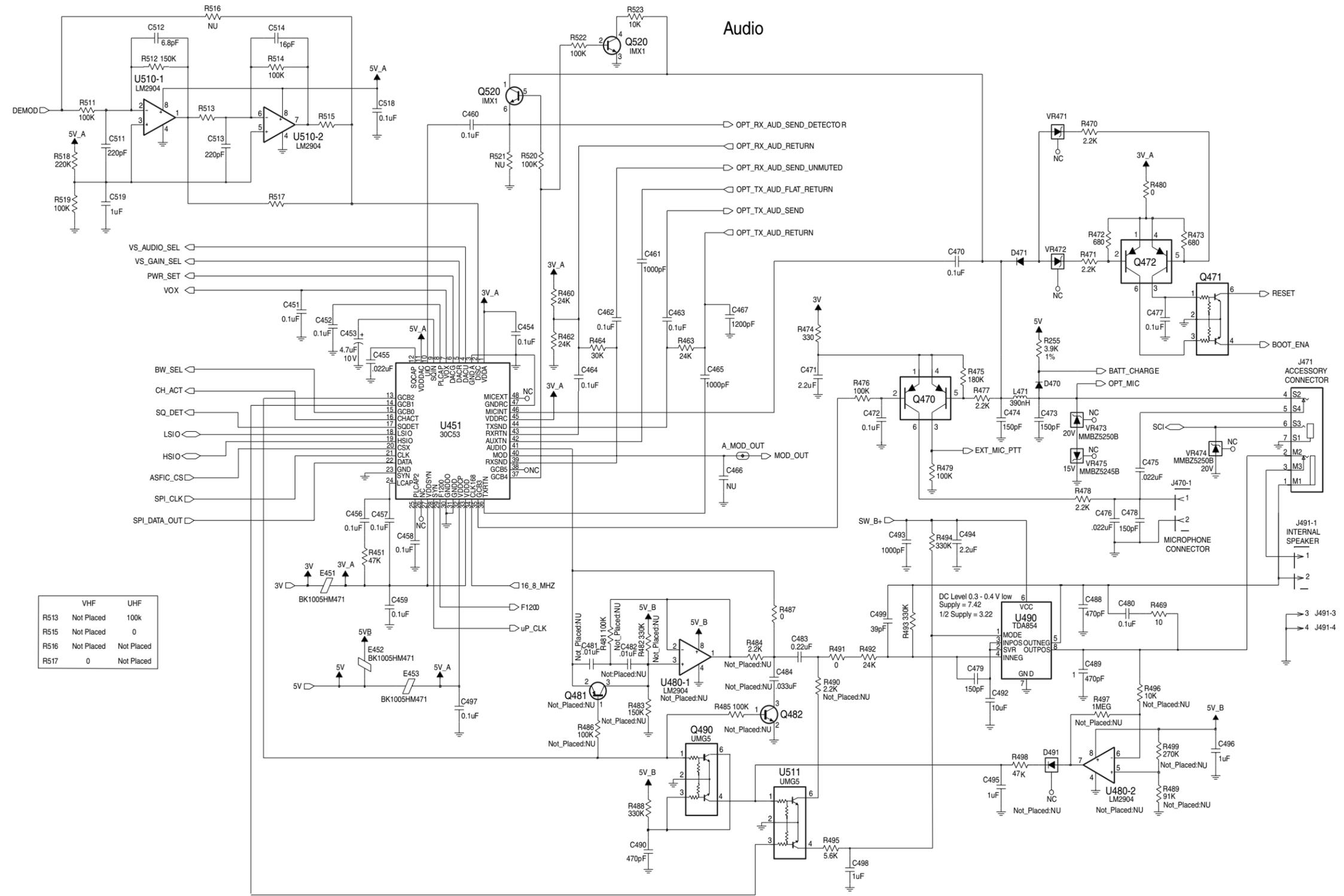
Figure 12-47. UHF (465-495 MHz) Audio Circuitry Schematic Diagram (8486634Z02-O)
