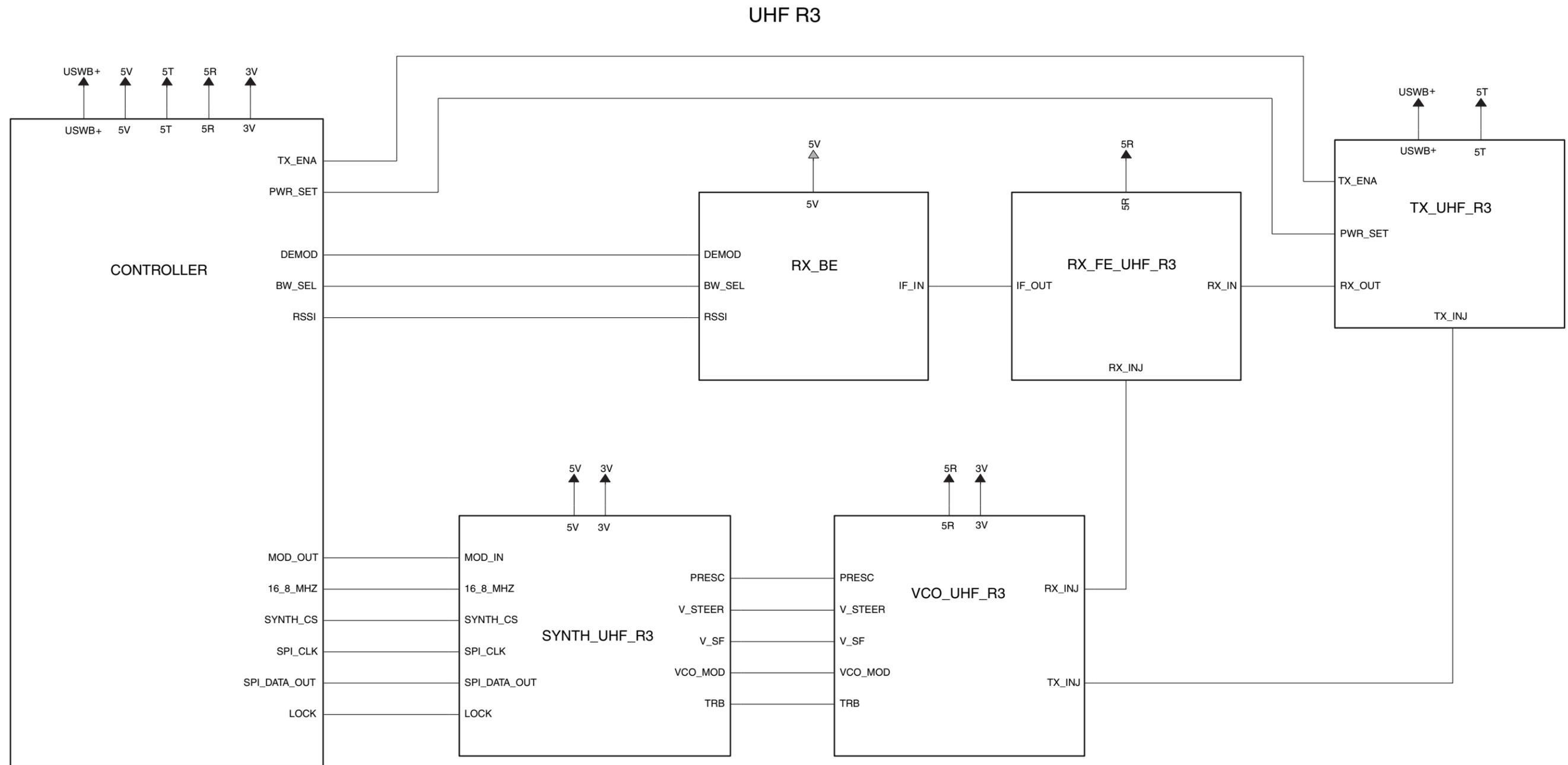
Figure 12-39. UHF (465-495 MHz) Radio Circuit Block Diagram (8486634Z02-O)
