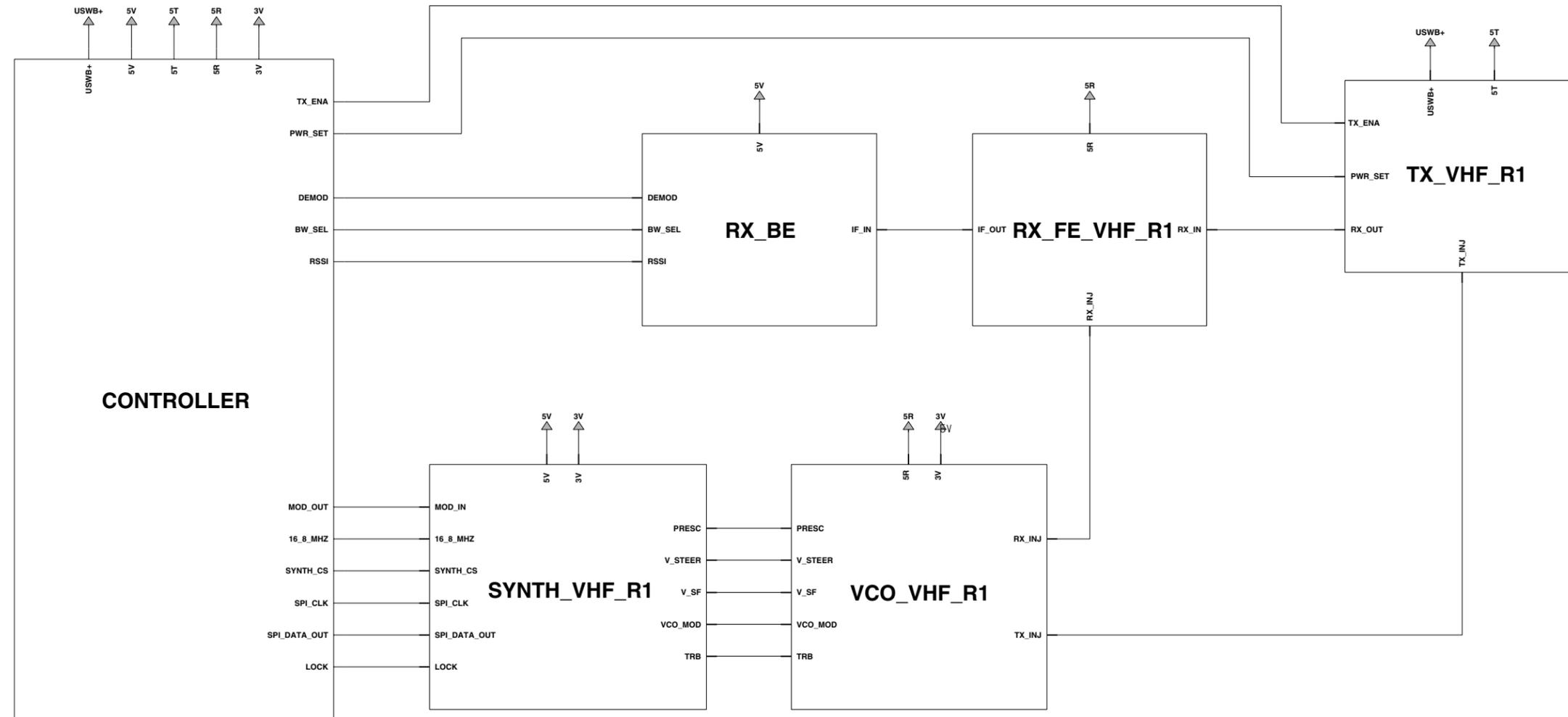
Figure 7-15. VHF (136-162 MHz) Radio Circuit Block Interconnect Diagram (8486769Z04-C)
