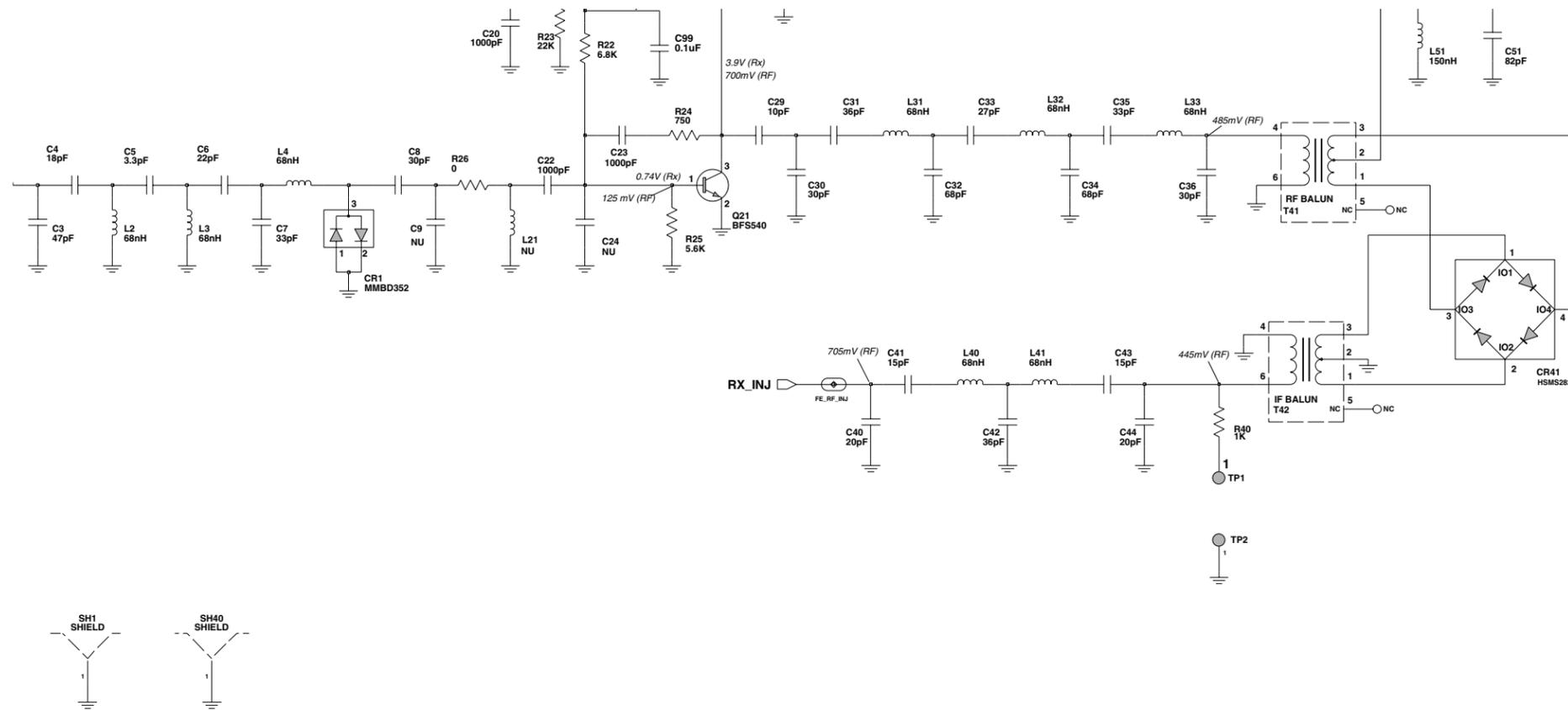
Figure 7-16. VHF (136-162 MHz) Receiver Front End Schematic Diagram (8486769Z04-C)
