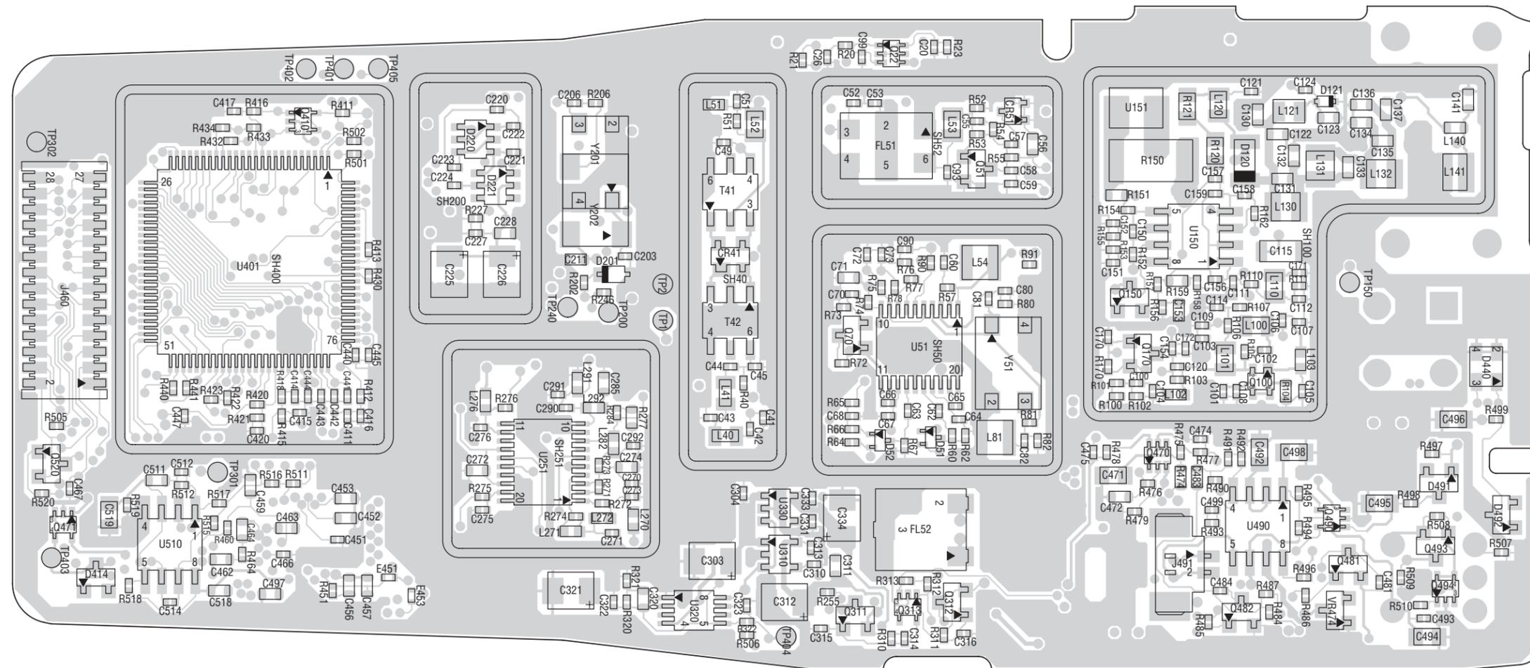
Figure 12-26. UHF (438-470 MHz) Board Solder Side View (8486348Z09-A)
