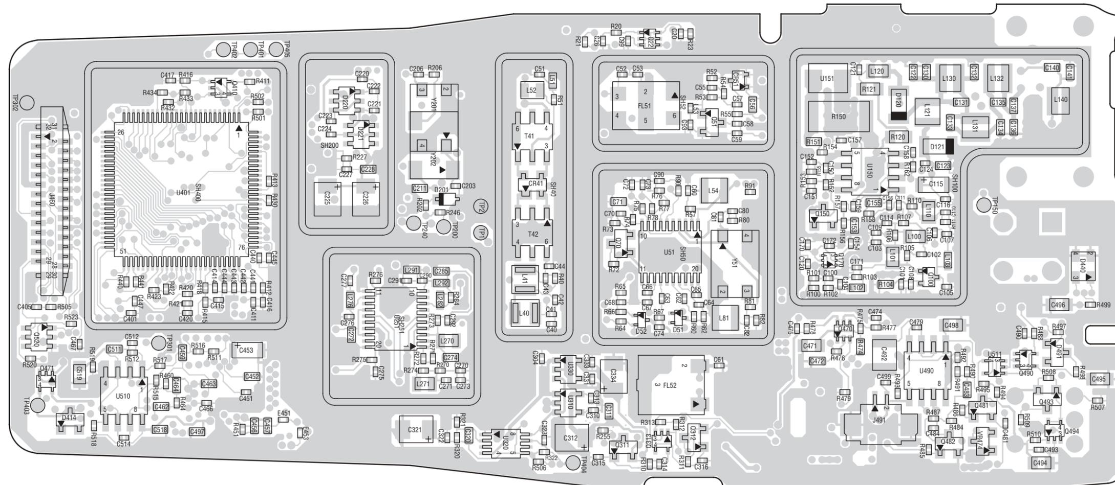
Figure 7-50. VHF (146-174 MHz) Board Solder Side View (8486342Z13-C)
