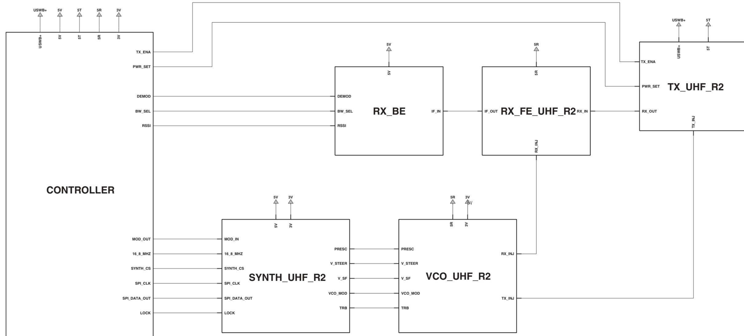
Figure 12-15. UHF (438-470 MHz) Radio Circuit Block Diagram (8486348Z09-A)
