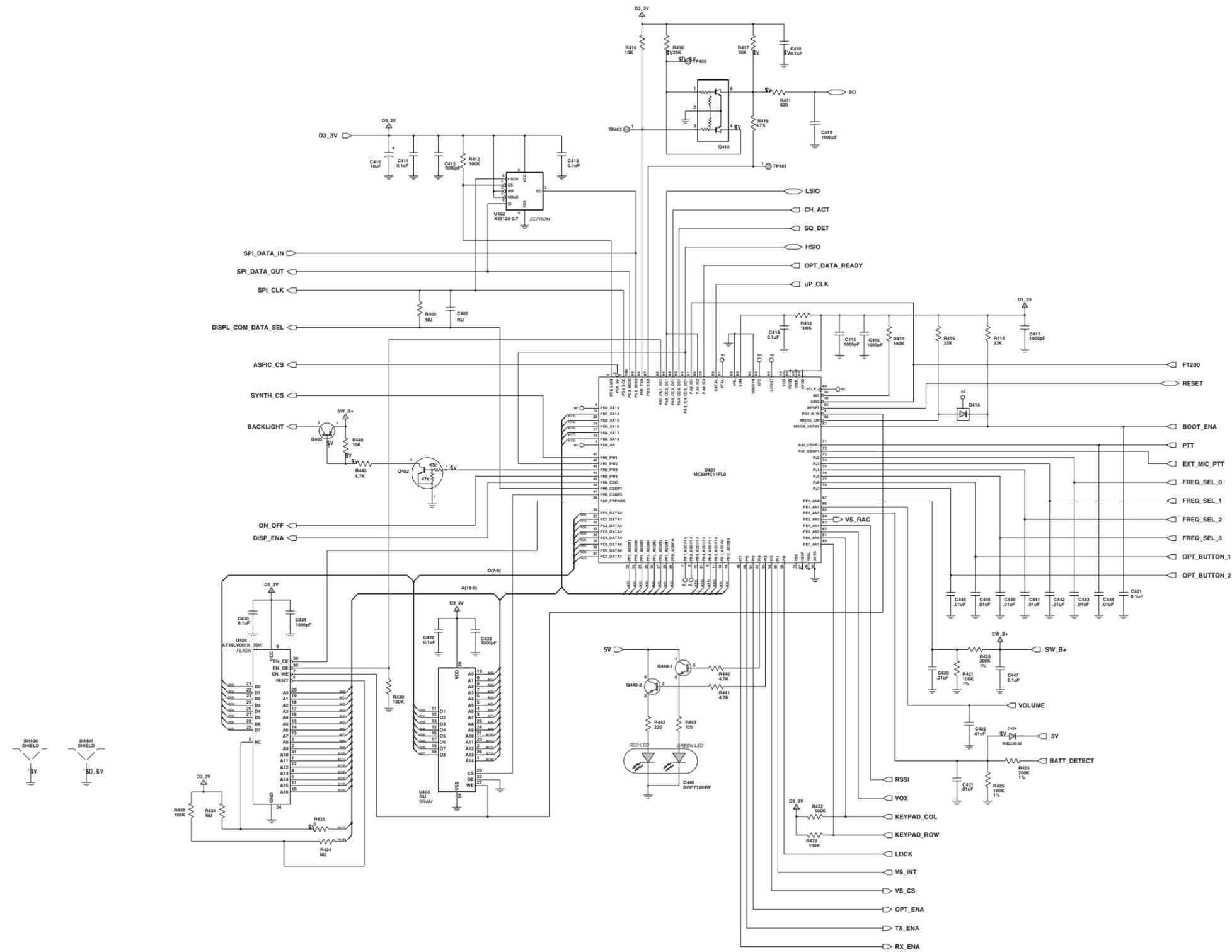
Figure 12-34. UHF (438-470 MHz) Microprocessor Circuitry Schematic Diagram (8486348Z13-C)
