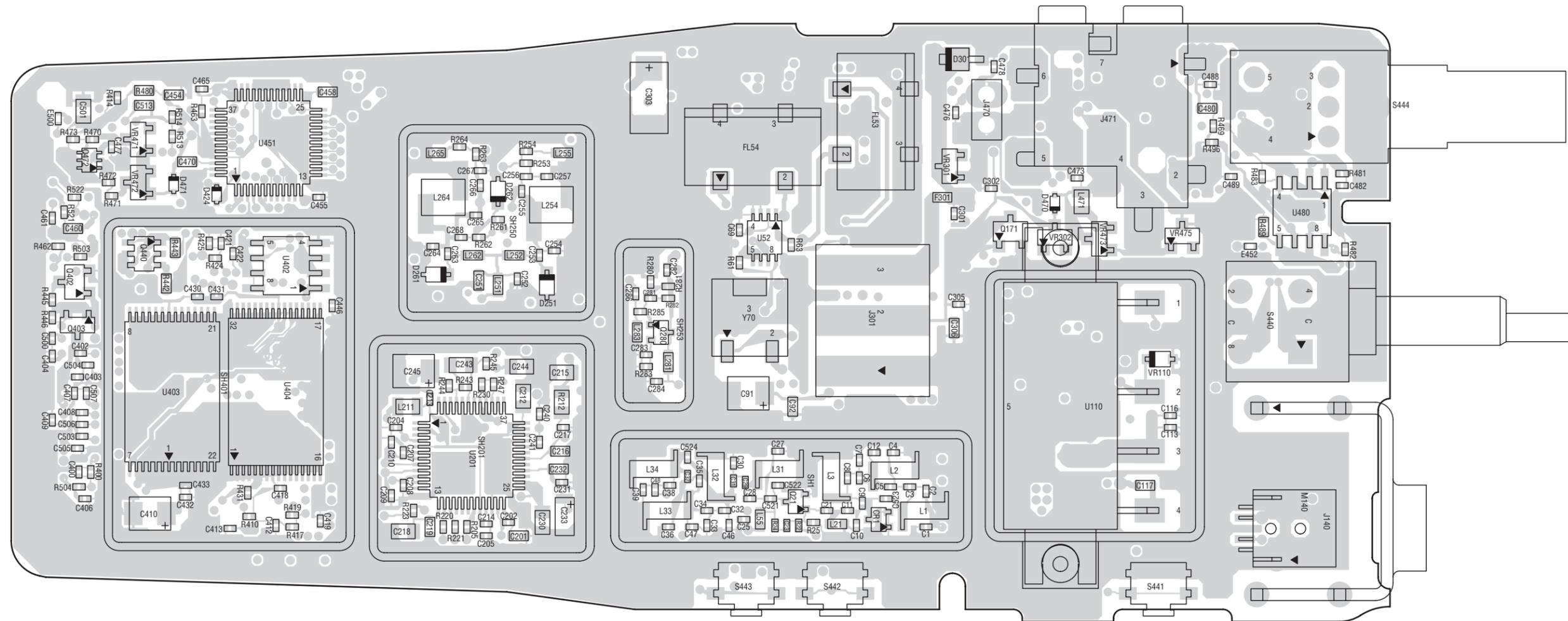
Figure 12-37. UHF (438-470 MHz) Board Component Side View (8486348Z13-C)
