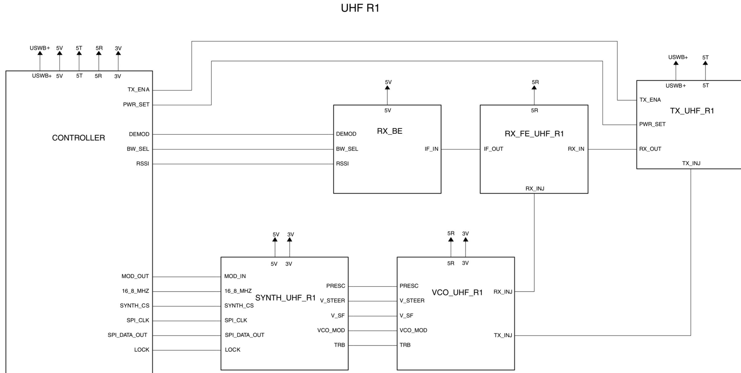
Figure 12-3. UHF (403-440 MHz) Radio Circuit Block Diagram (8486635Z03-O)
