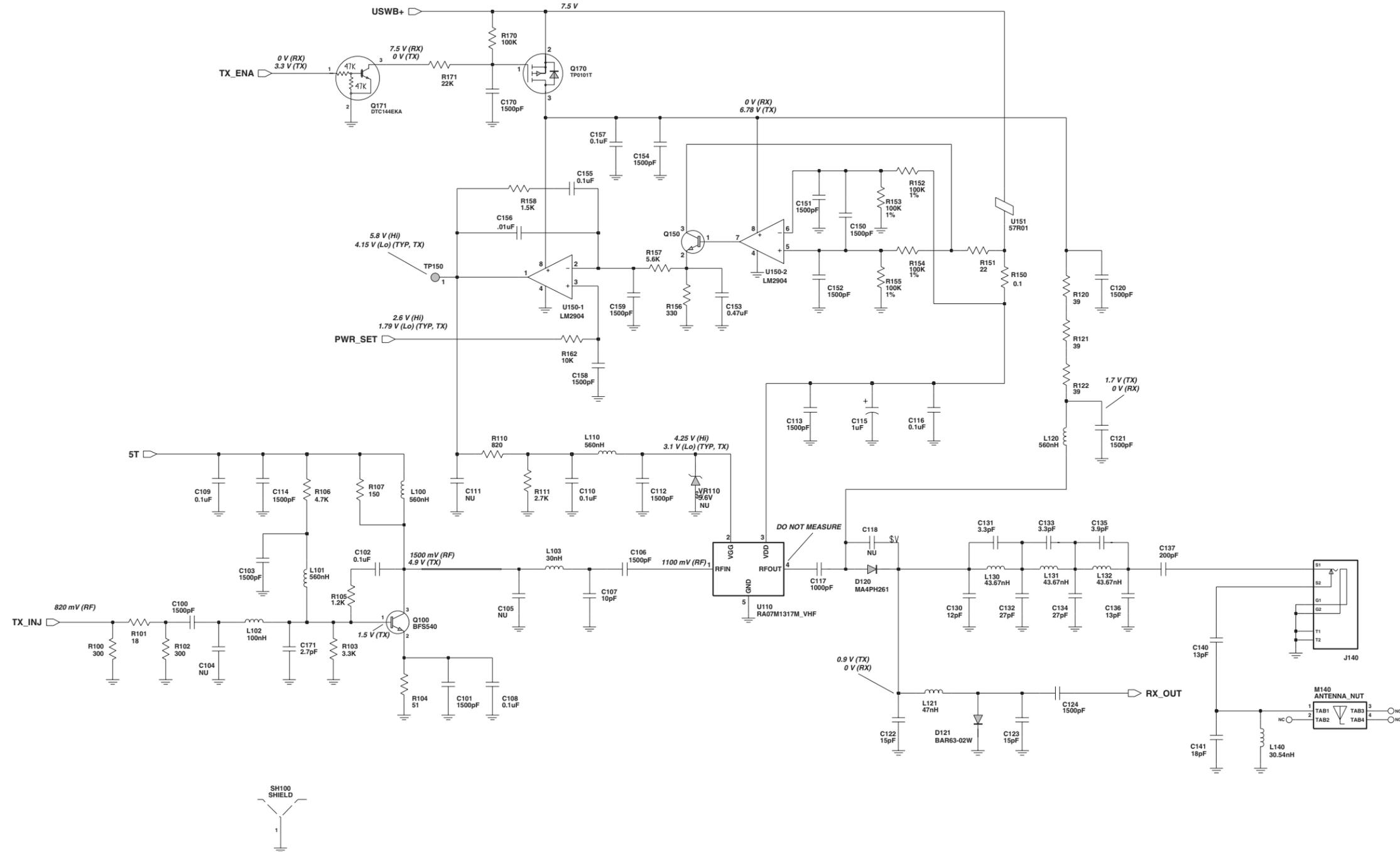
Figure 7-32. VHF (146-174 MHz) Transmitter and Power Control Schematic Diagram (8486342Z09-A)
