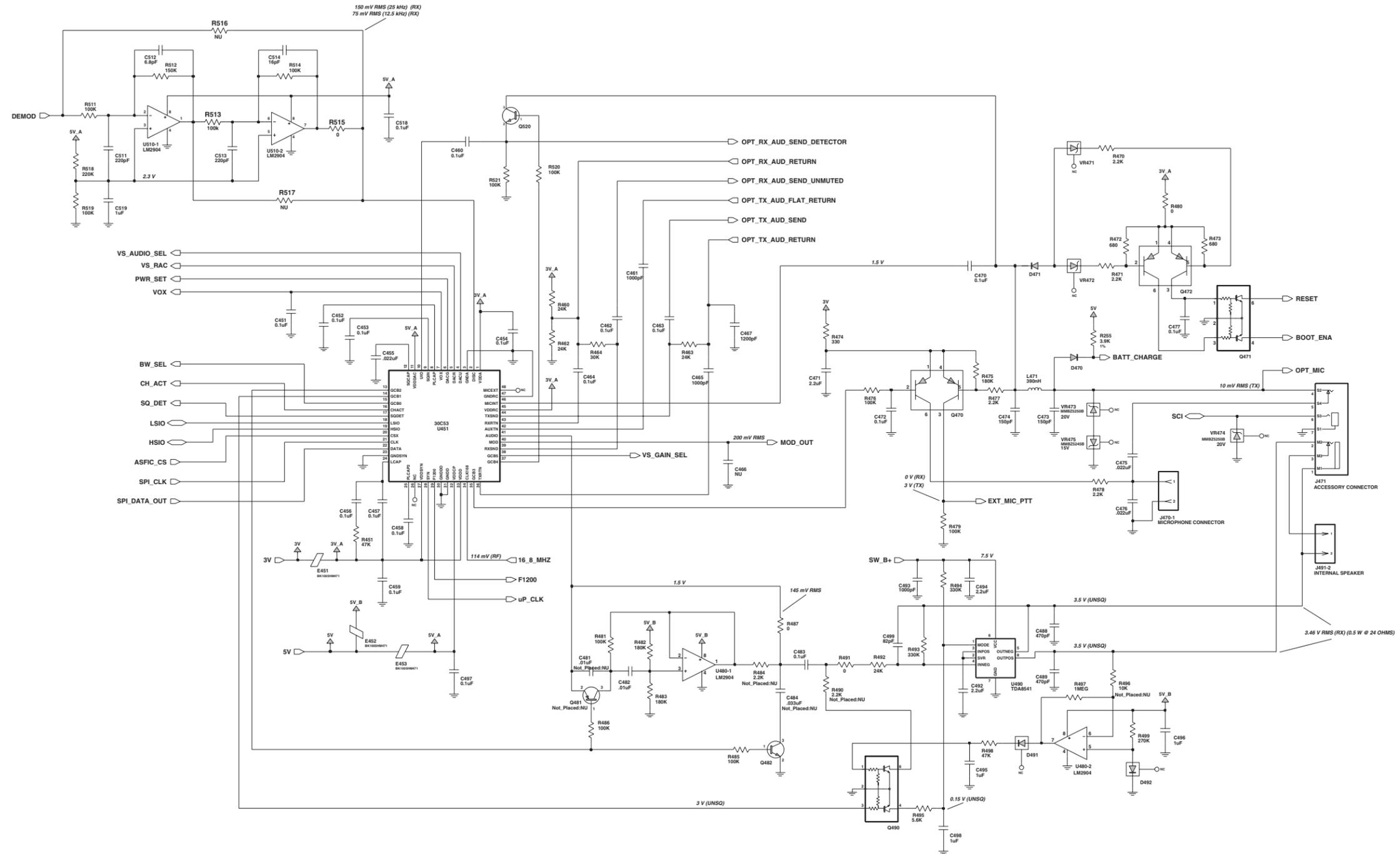
Figure 12-23. UHF (438-470 MHz) Audio Circuitry Schematic Diagram (8486348Z09-A)
