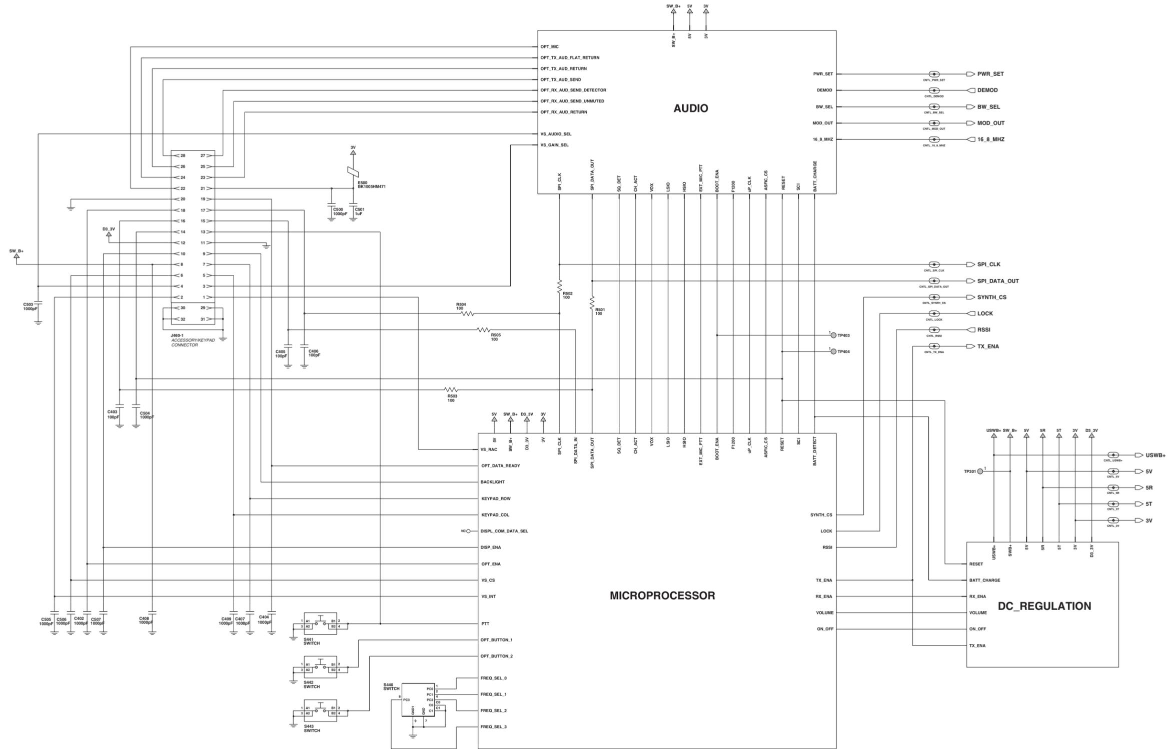
Figure 7-9. VHF (136-162 MHz) Controller Interconnect Schematic Diagram (8486769Z02-A)
