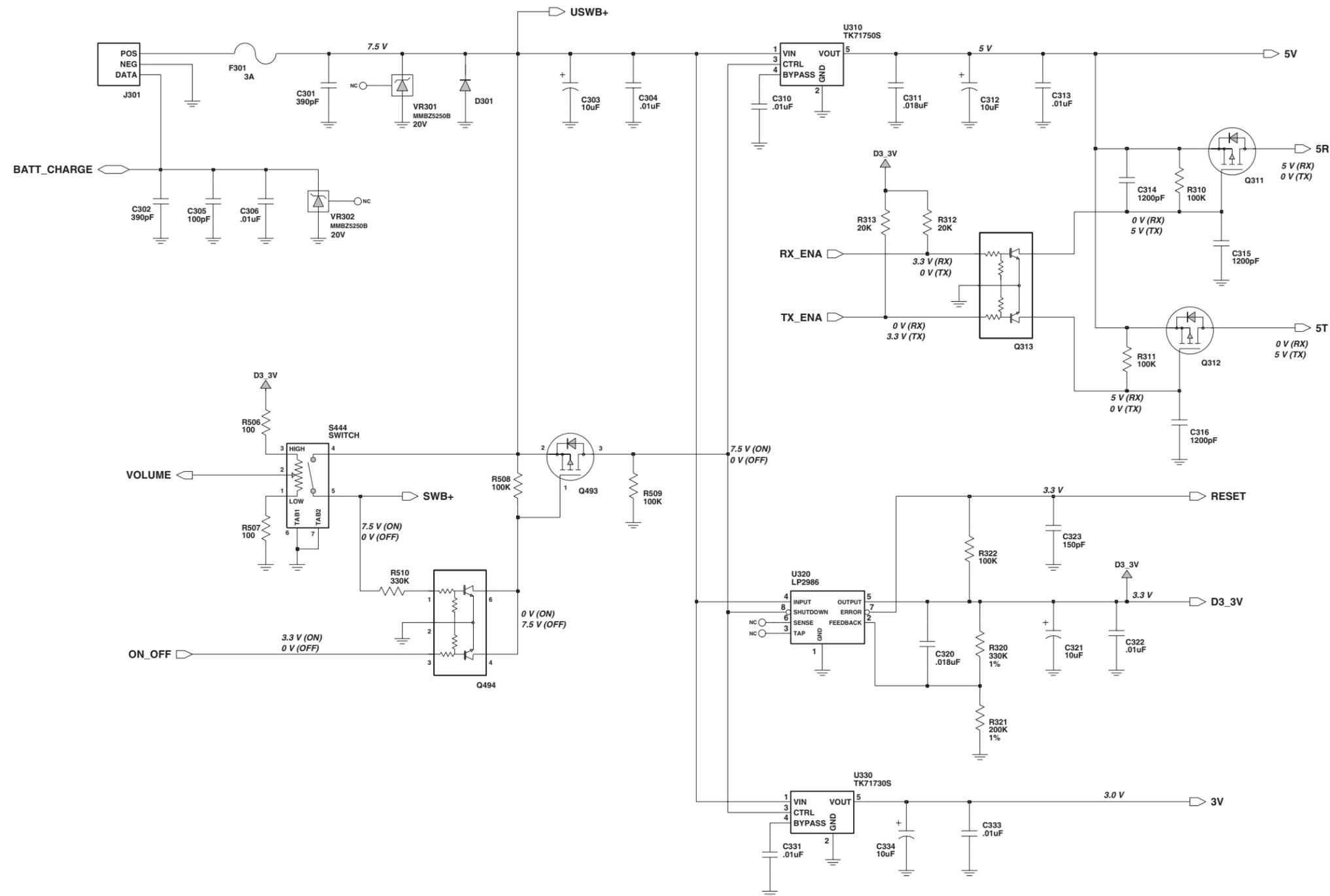
Figure 12-24. UHF (438-470 MHz) DC Regulation Schematic Diagram (8486348Z09-A)
