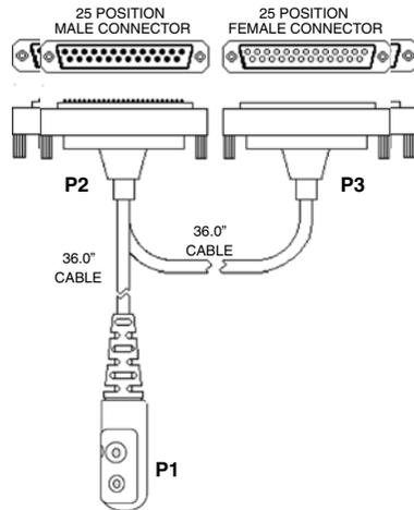
Figure 1-1. Programming/Test Cable
