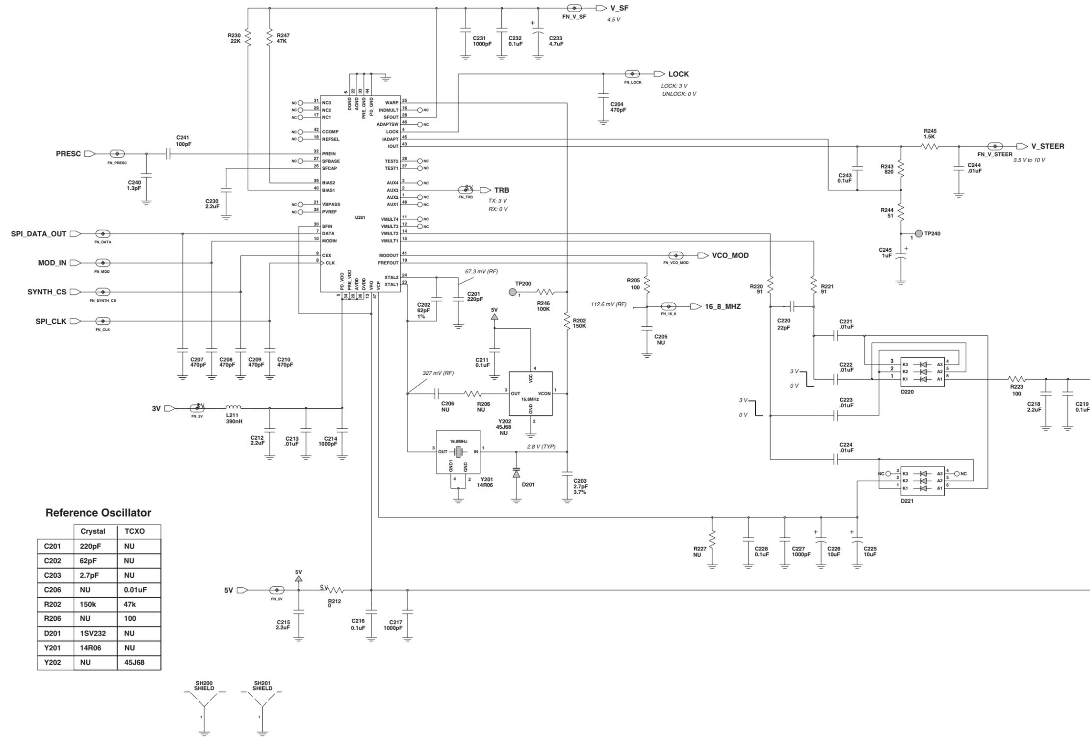
Figure 12-30. UHF (438-470 MHz) Synthesizer Schematic Diagram (8486348Z13-C)
