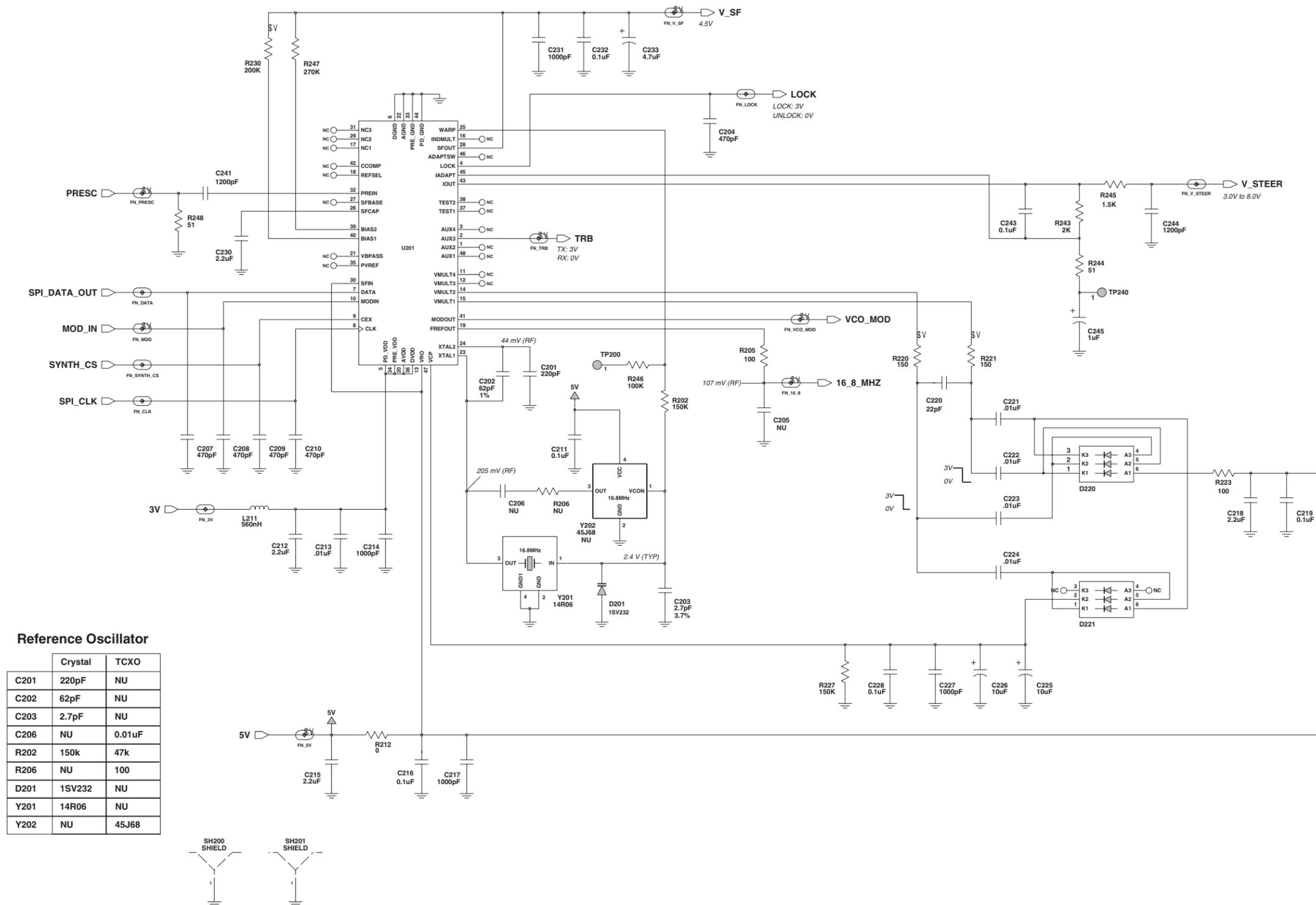
Figure 7-42. VHF (146-174 MHz) Synthesizer Schematic Diagram (8486342Z13-C)
