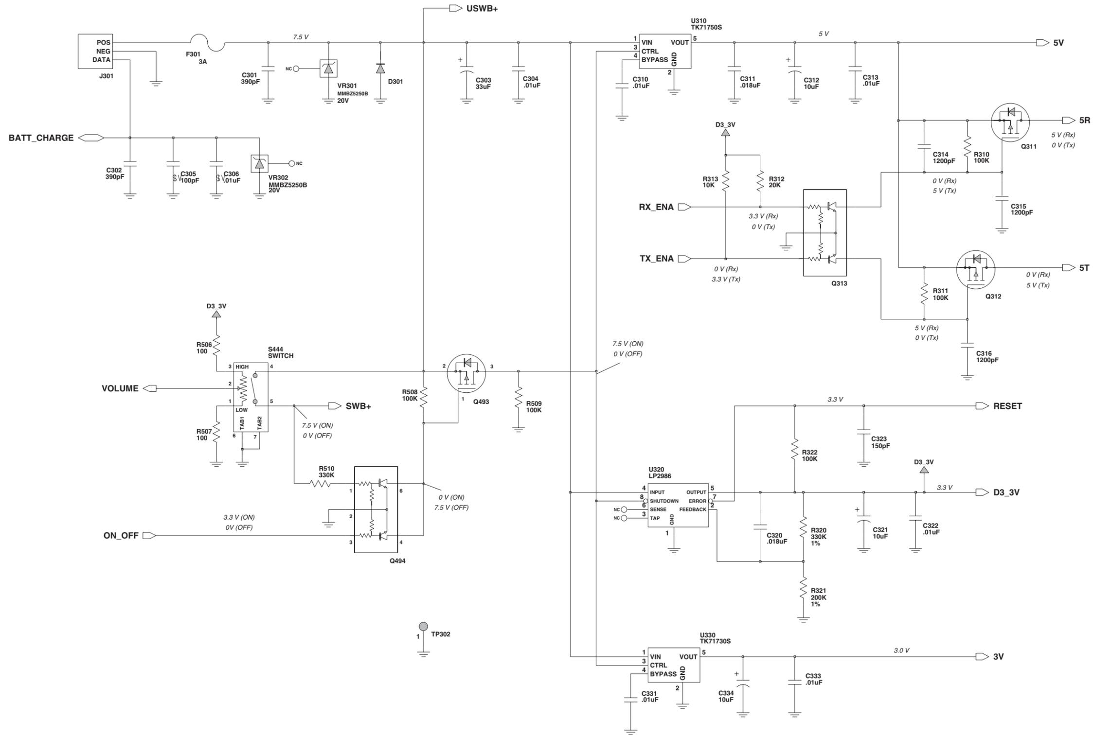
Figure 12-36. UHF (438-470 MHz) DC Regulation Schematic Diagram (8486348Z13-C)
