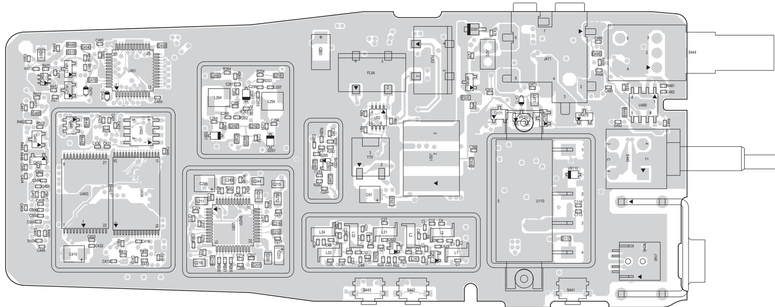
Figure 12-49. UHF (465-495 MHz) Board Component Side View (8486634Z02-O)
