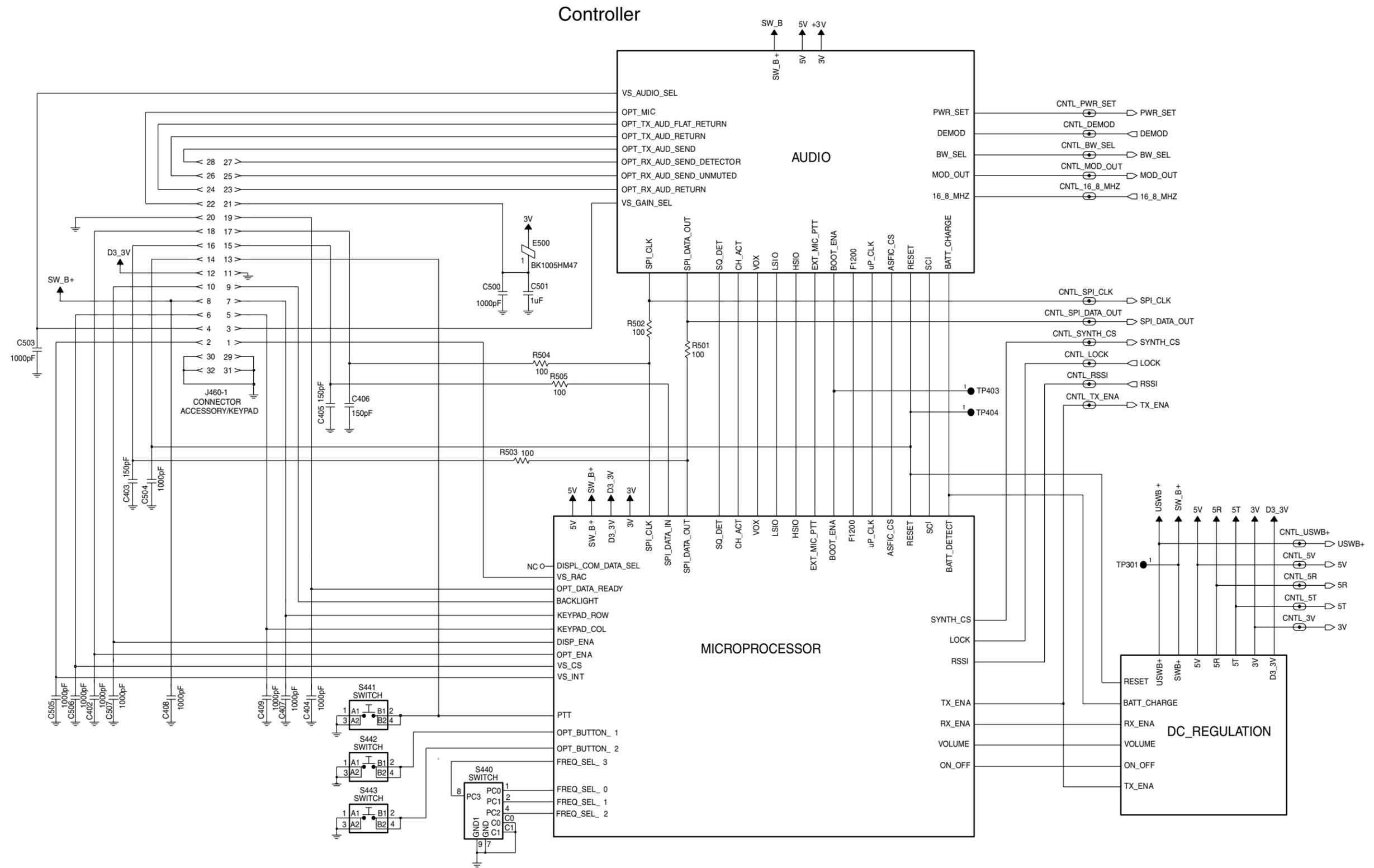
Figure 12-45. UHF (465-495 MHz) Controller Interconnect Schematic Diagram (8486634Z02-O)
