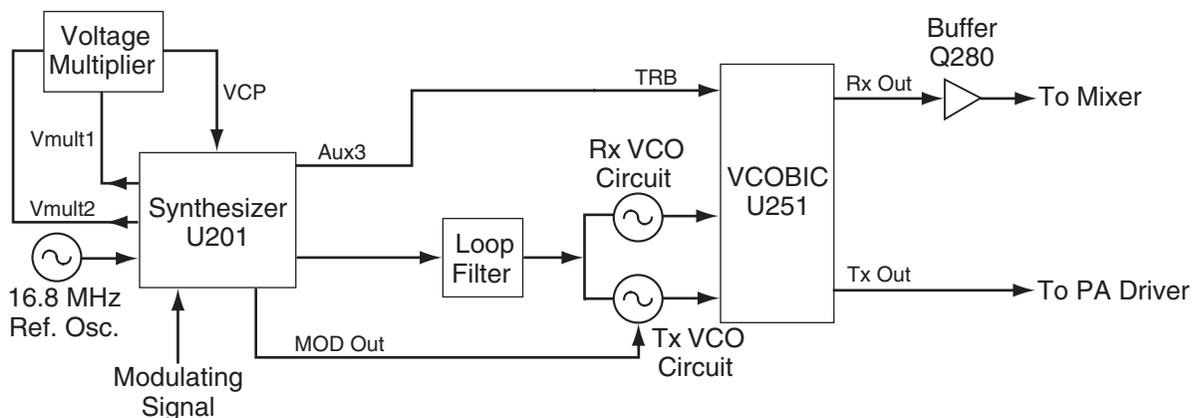
Figure 8-3. UHF Frequency Generation Unit Block Diagram
