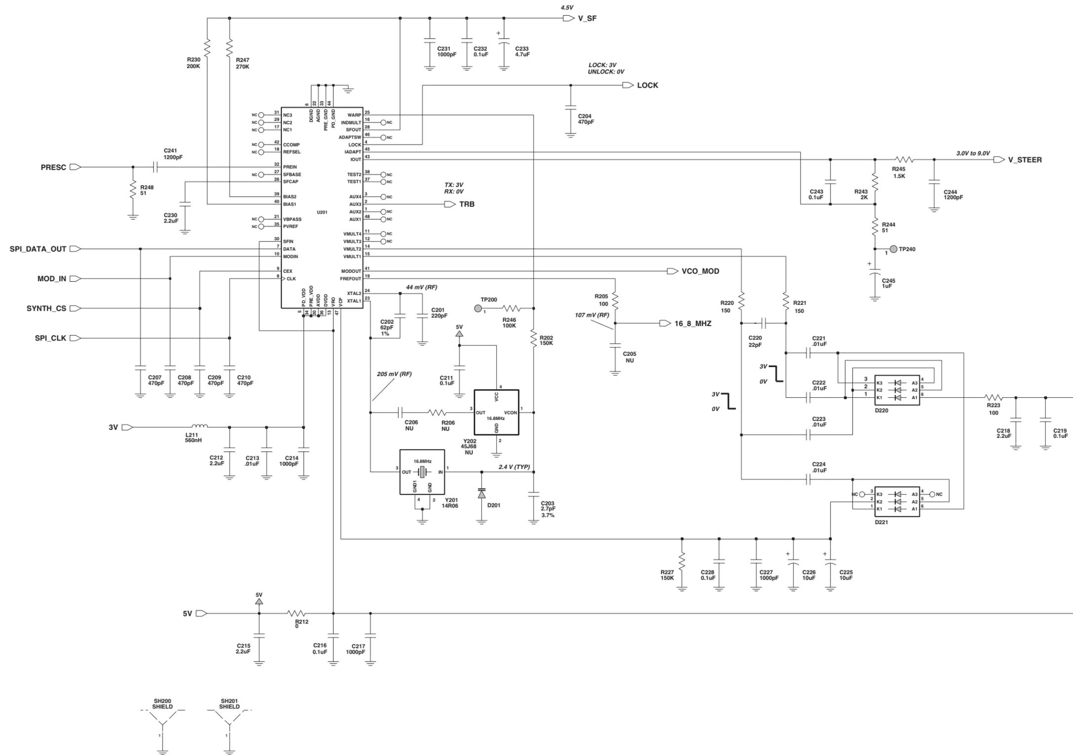
Figure 7-30. VHF (146-174 MHz) Synthesizer Schematic Diagram (8486342Z09-A)
