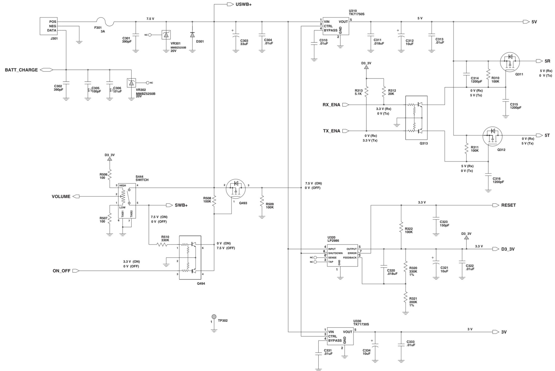
Figure 7-24. VHF (136-162 MHz) DC Regulation Schematic Diagram (8486769Z04-C)
