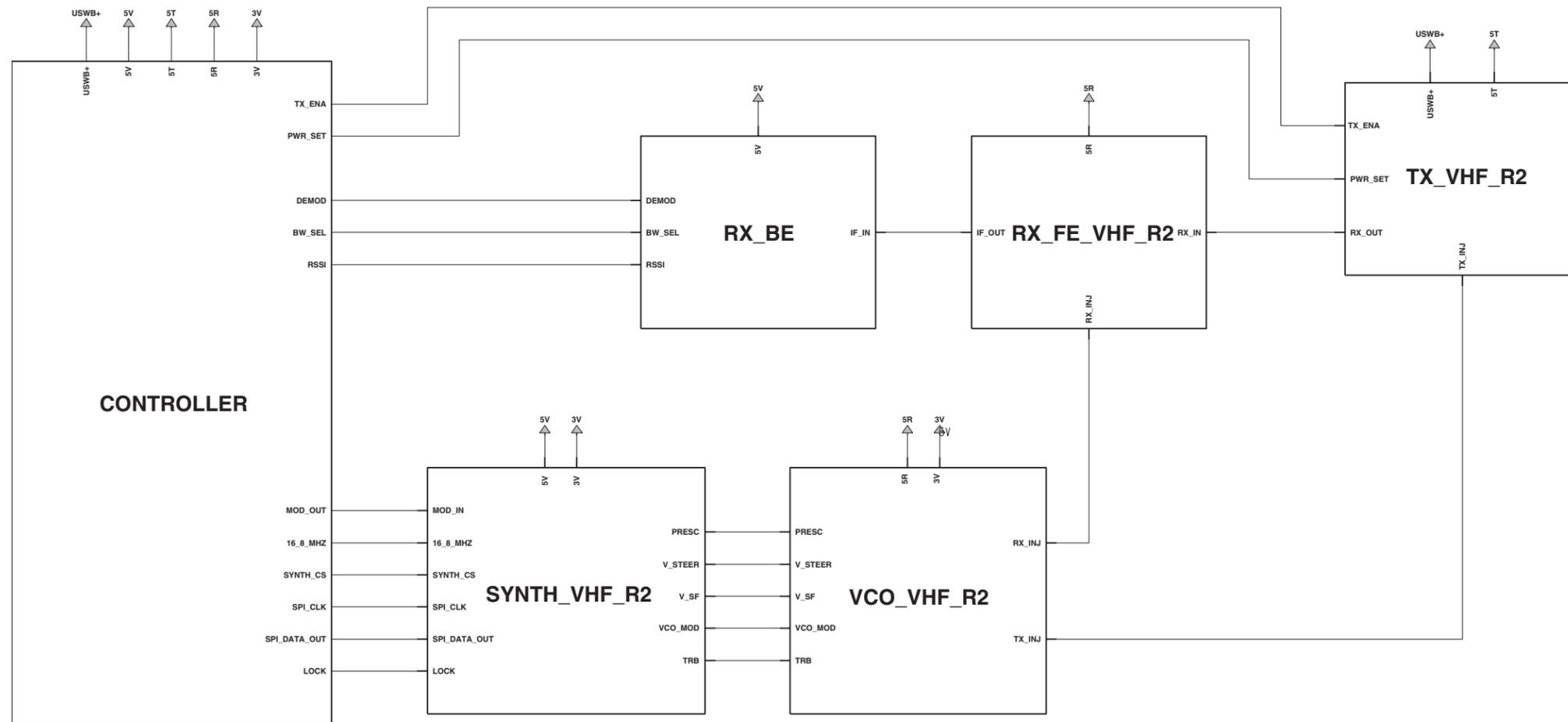
Figure 7-27. VHF (146-174 MHz) Radio Circuit Block Interconnect Diagram (8486342Z09-A)
