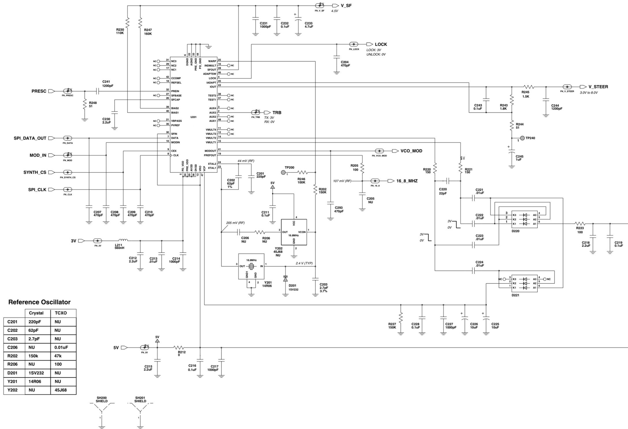
Figure 7-18. VHF (136-162 MHz) Synthesizer Schematic Diagram (8486769Z04-C)
