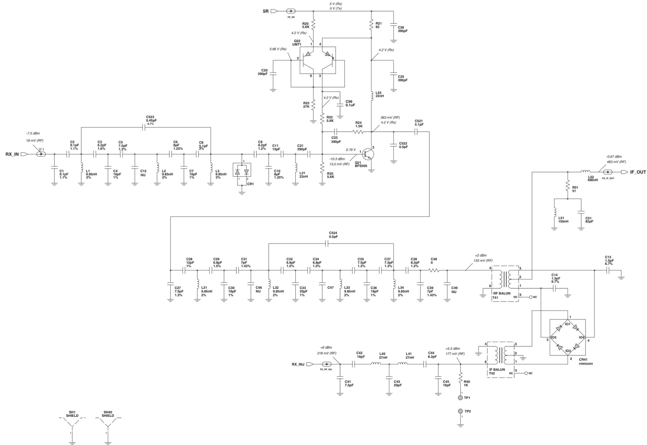
Figure 12-28. UHF (438-470 MHz) Receiver Front End Schematic Diagram (8486348Z13-C)
