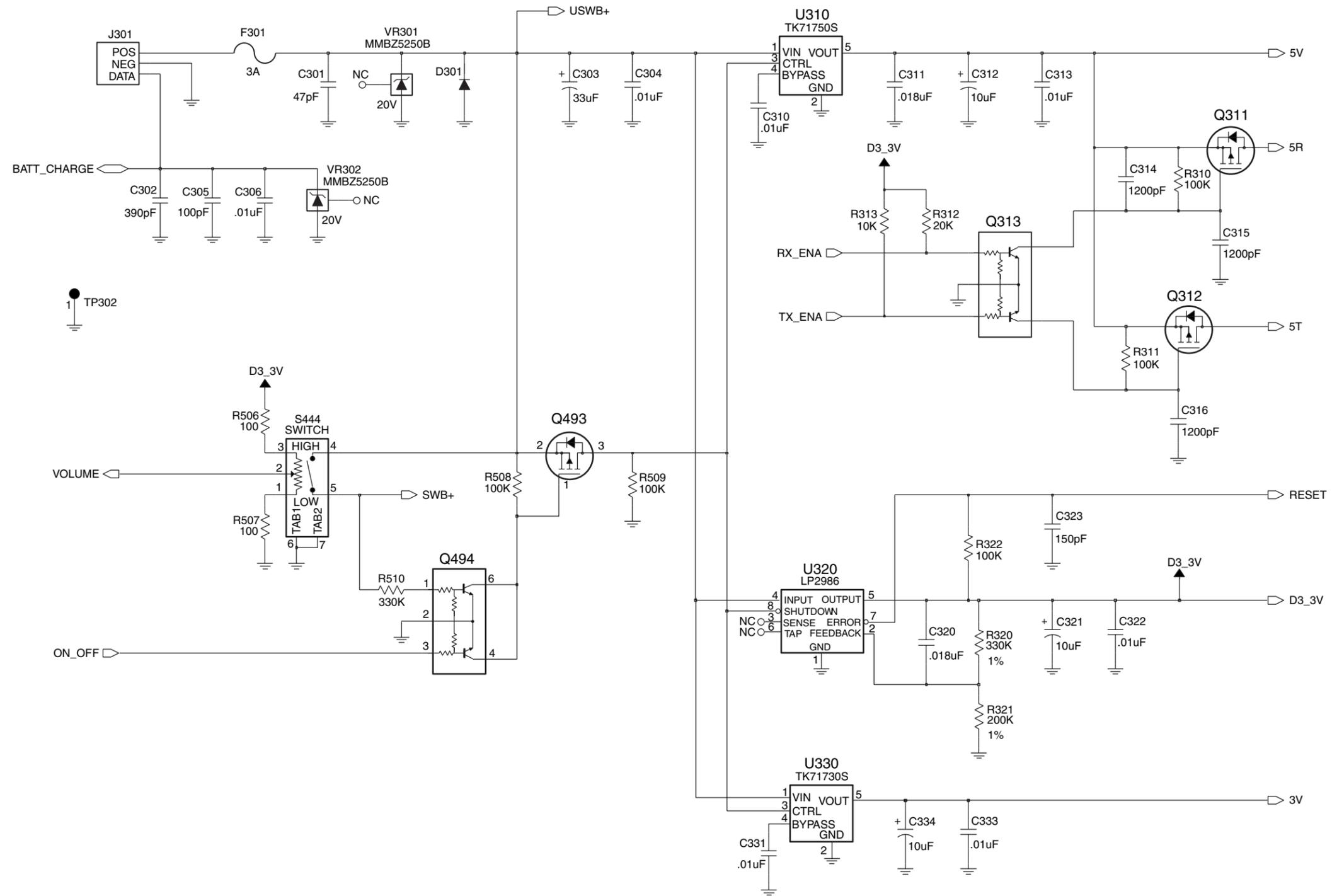
Figure 12-12. UHF (403-440 MHz) DC Regulation Schematic Diagram (8486635Z03-O)
