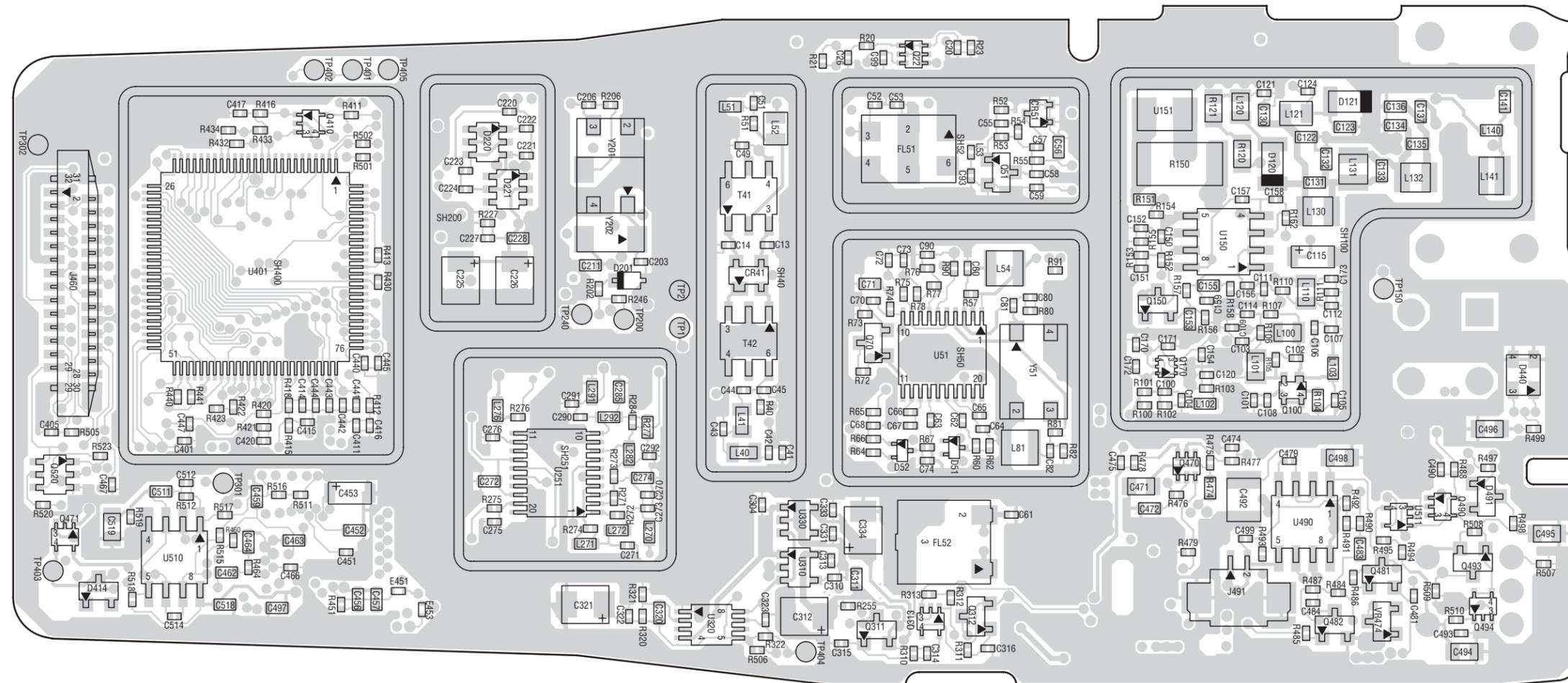
Figure 12-38. UHF (438-470 MHz) Board Solder Side View (8486348Z13-C)
