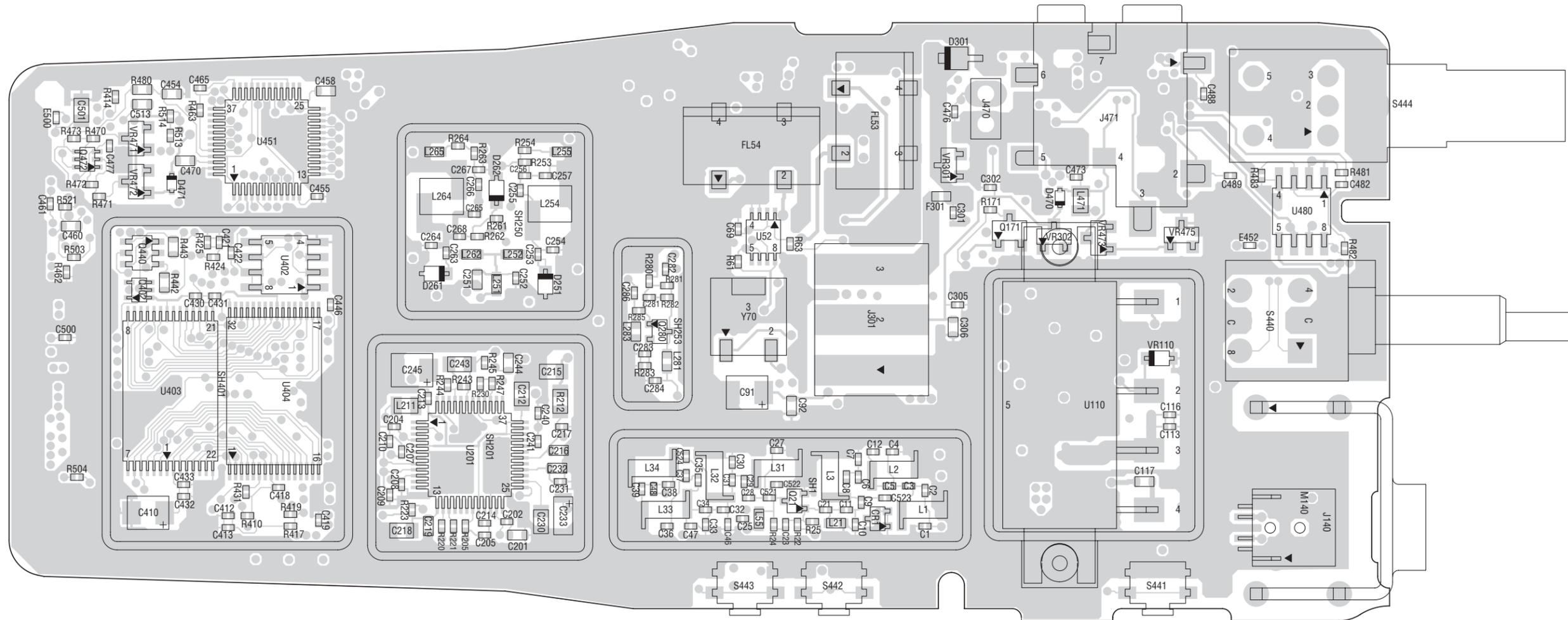
Figure 12-25. UHF (438-470 MHz) Board Component Side View (8486348Z09-A)
