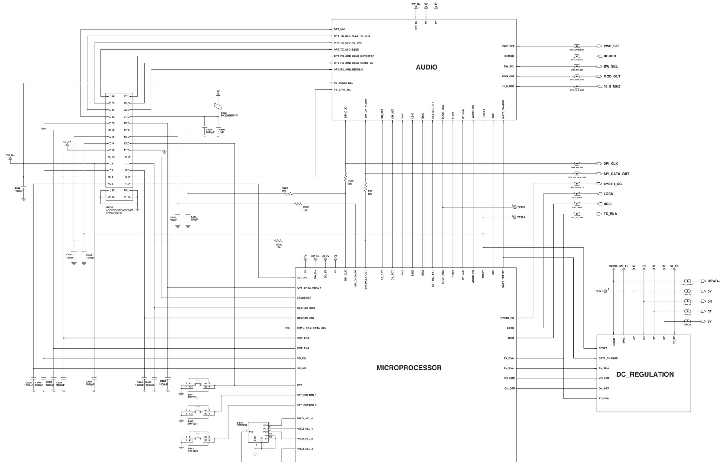
Figure 7-21. VHF (136-162 MHz) Controller Interconnect Schematic Diagram (8486769Z04-C)
