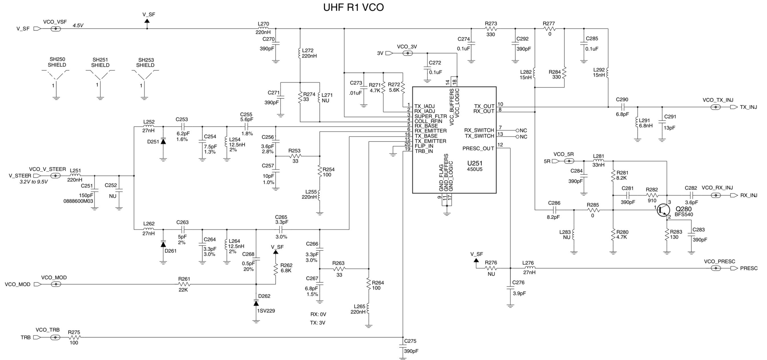
Figure 12-7. UHF (403-440 MHz) Voltage Controlled Oscillator Schematic Diagram (8486635Z03-O)
