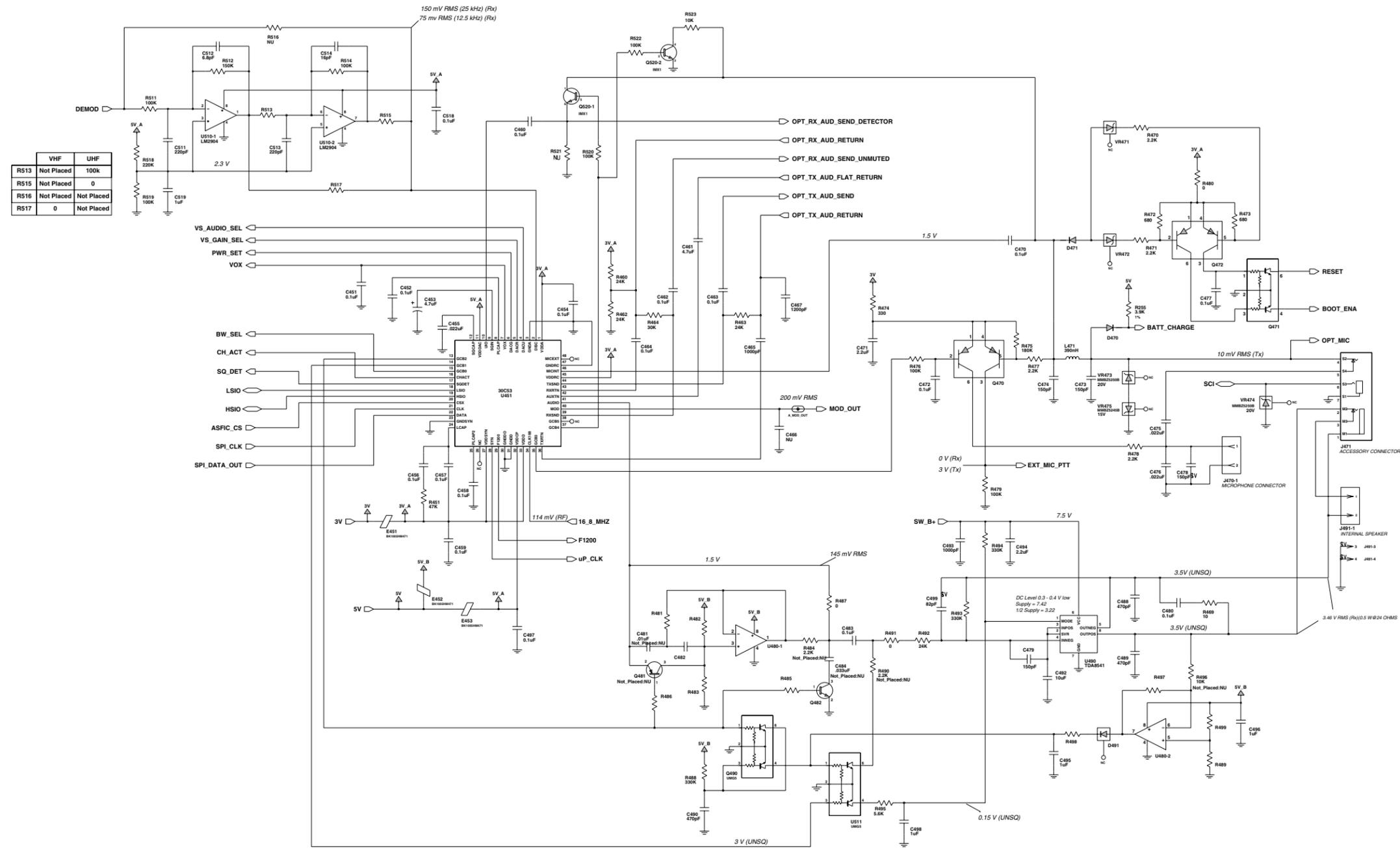
Figure 7-11. VHF (136-162 MHz) Audio Circuitry Schematic Diagram (8486769Z02-A)
