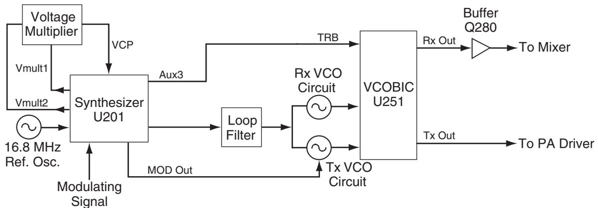
Figure 9-3. UHF Frequency Generation Unit Block Diagram
