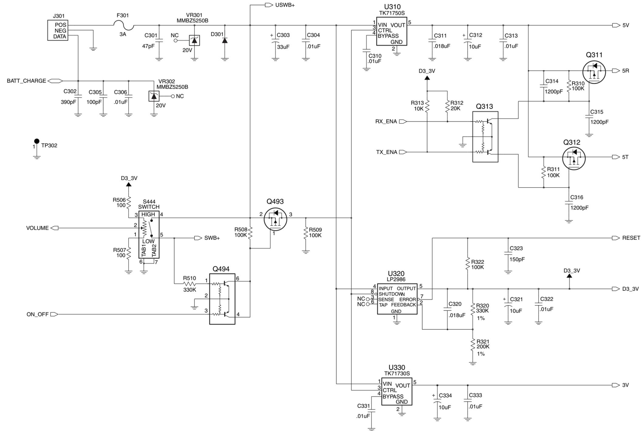
Figure 12-48. UHF (465-495 MHz) DC Regulation Schematic Diagram (8486634Z02-O)
