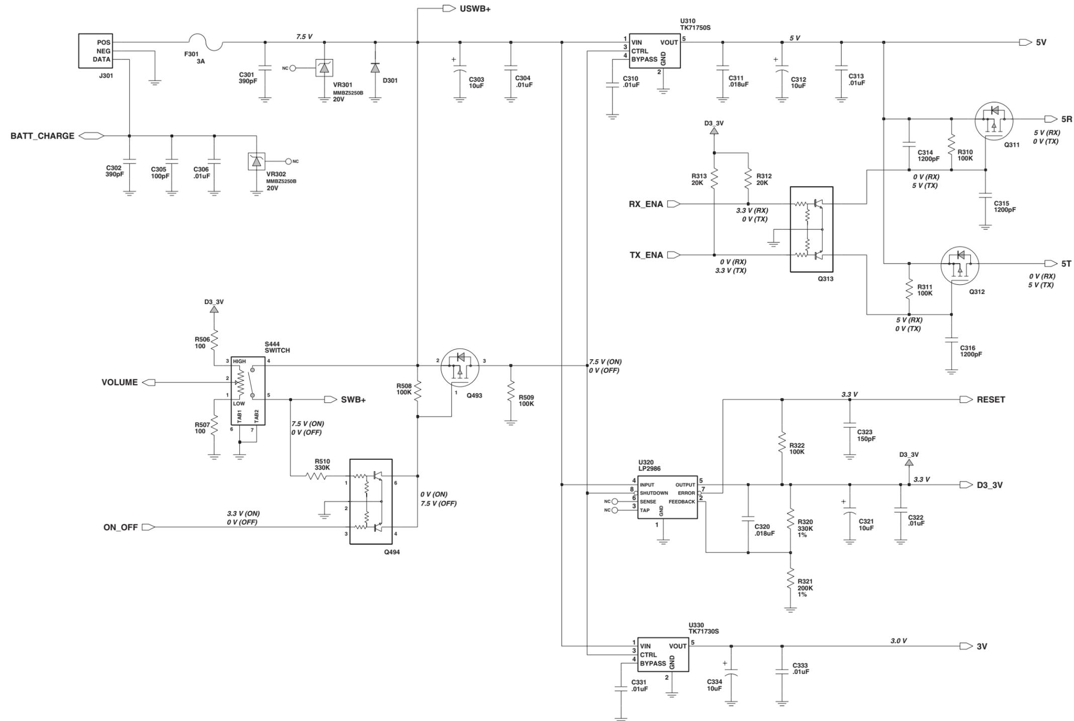
Figure 7-36. VHF (146-174 MHz) DC Regulation Schematic Diagram (8486342Z09-A)
