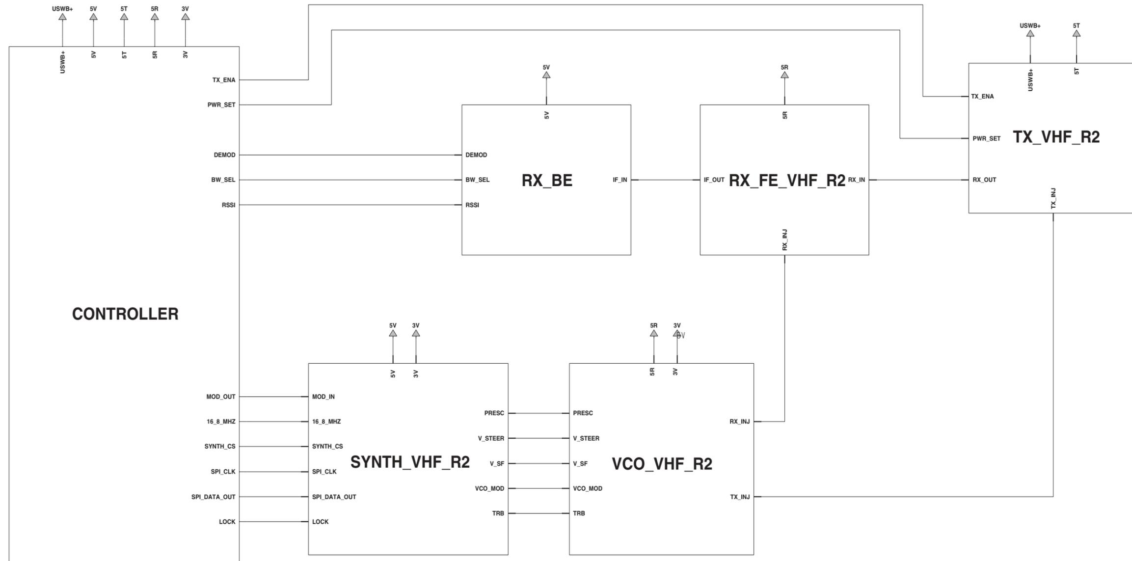
Figure 7-52. VHF (146-174 MHz) Radio Circuit Block Interconnect Diagram (8486769Z04-C)
