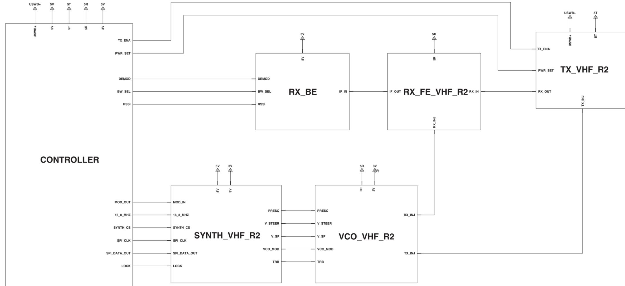
Figure 7-39. VHF (146-174 MHz) Radio Circuit Block Interconnect Diagram (8486342Z13-C)
