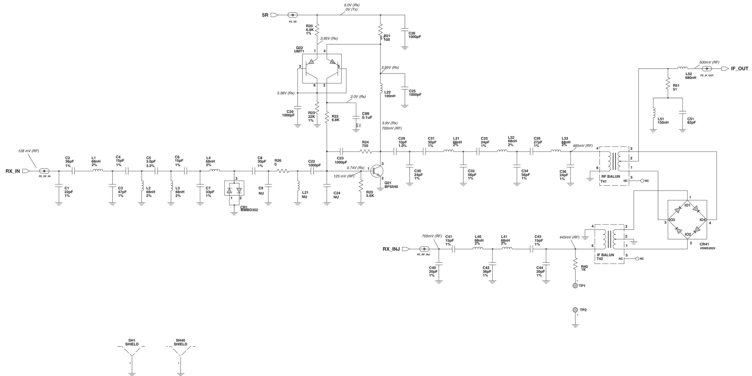
Figure 7-53. VHF (146-174 MHz) Receiver Front End Schematic Diagram (8486769Z04-C)
