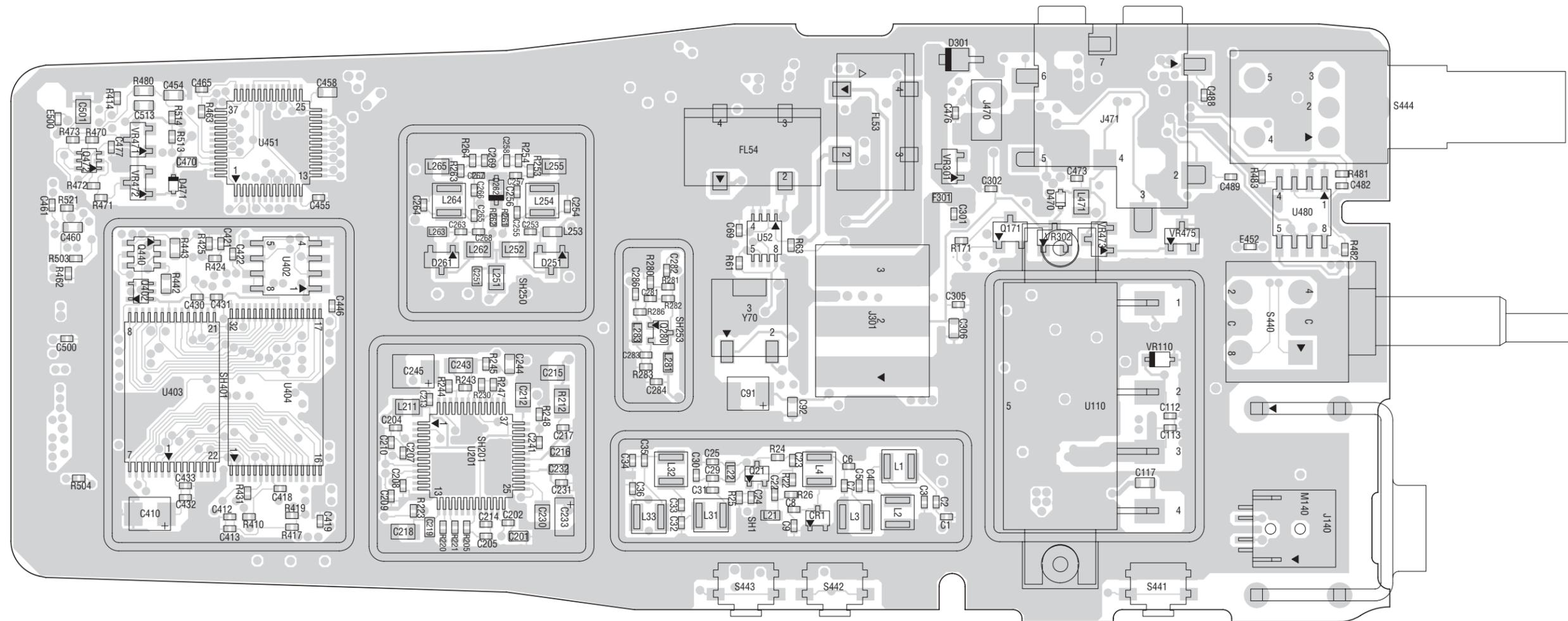
Figure 7-37. VHF (146-174 MHz) Board Component Side View (8486342Z09-A)
