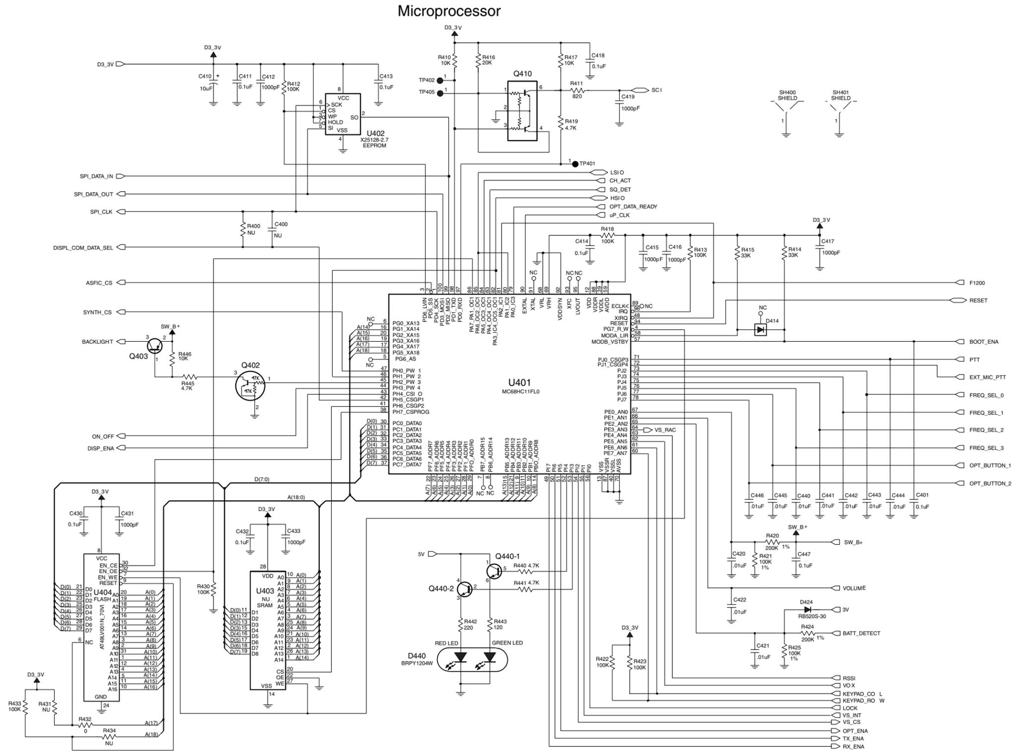
Figure 12-10. UHF (403-440 MHz) Microprocessor Circuitry Schematic Diagram (8486635Z03-O)
