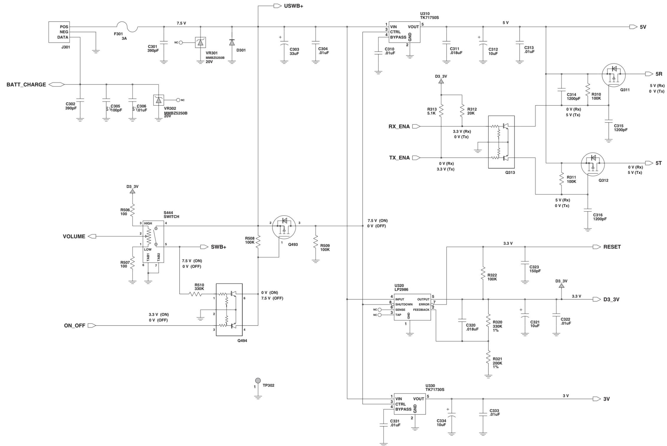
Figure 7-12. VHF (136-162 MHz) DC Regulation Schematic Diagram (8486769Z02-A)
