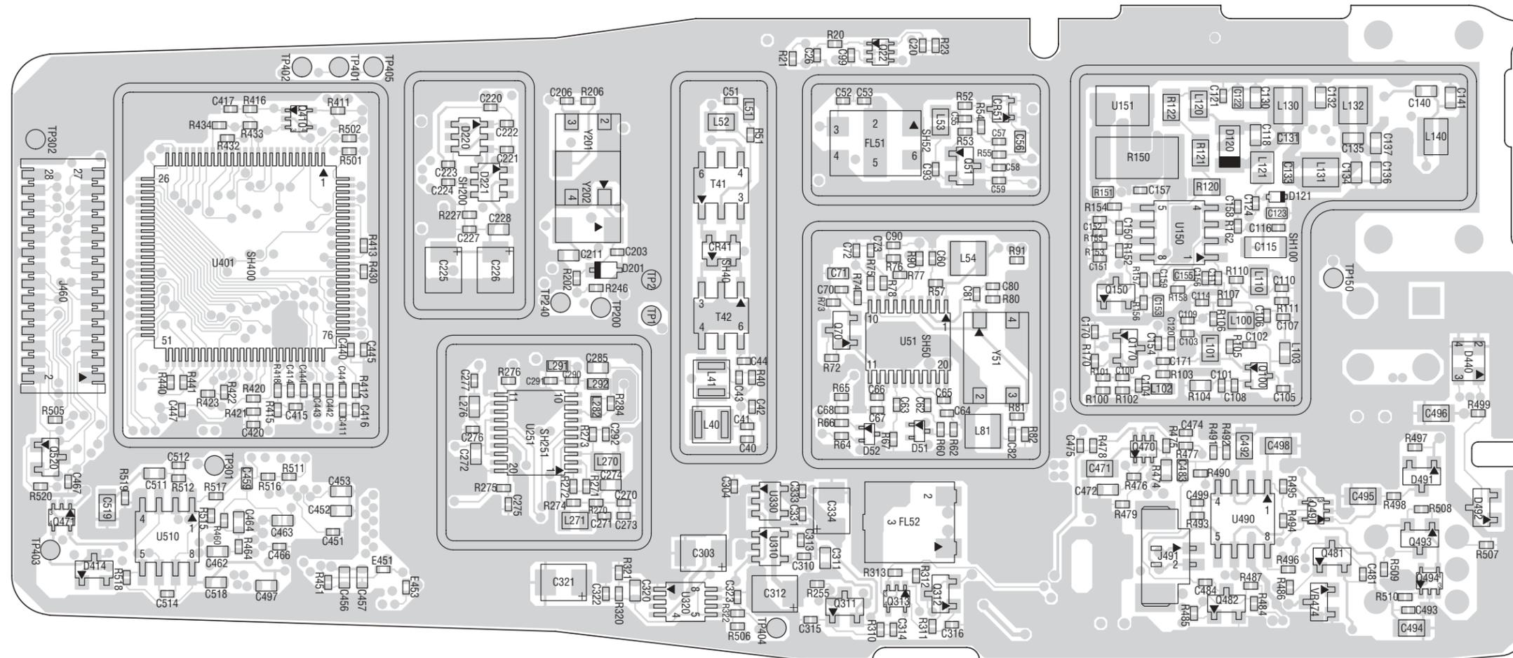
Figure 7-38. VHF (146-174 MHz) Board Solder Side View (8486342Z09-A)
