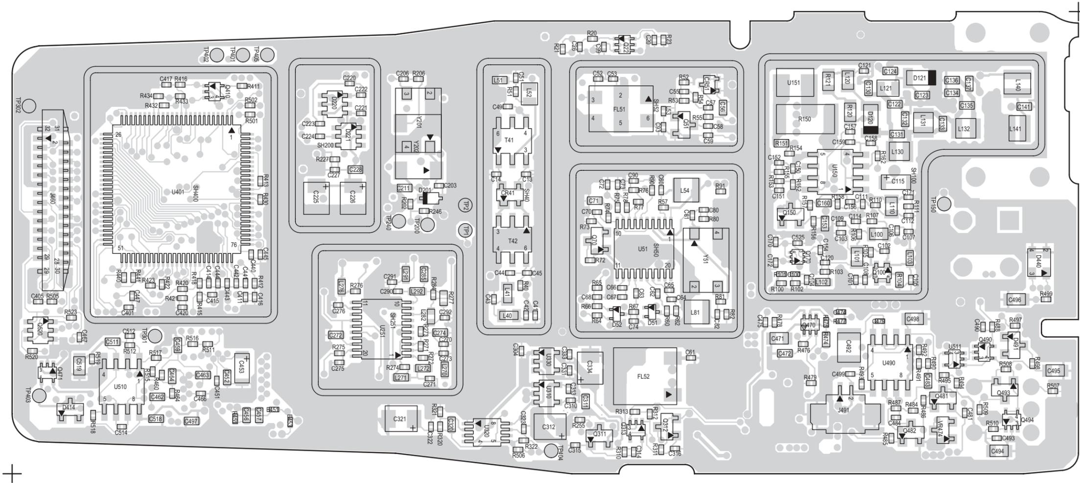
Figure 12-50. UHF (465-495 MHz) Board Solder Side View (8486634Z02-O)
