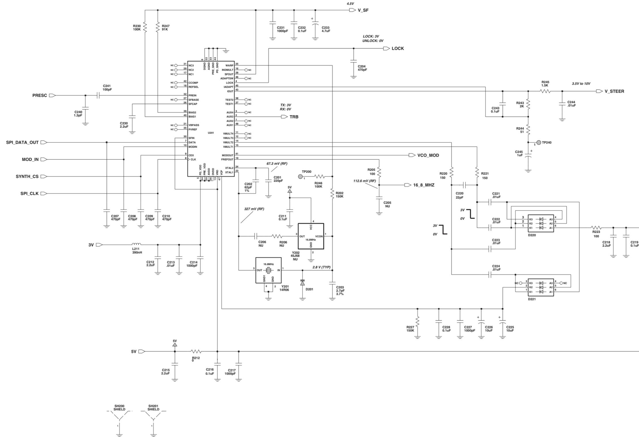
Figure 12-18. UHF (438-470 MHz) Synthesizer Schematic Diagram (8486348Z09-A)
