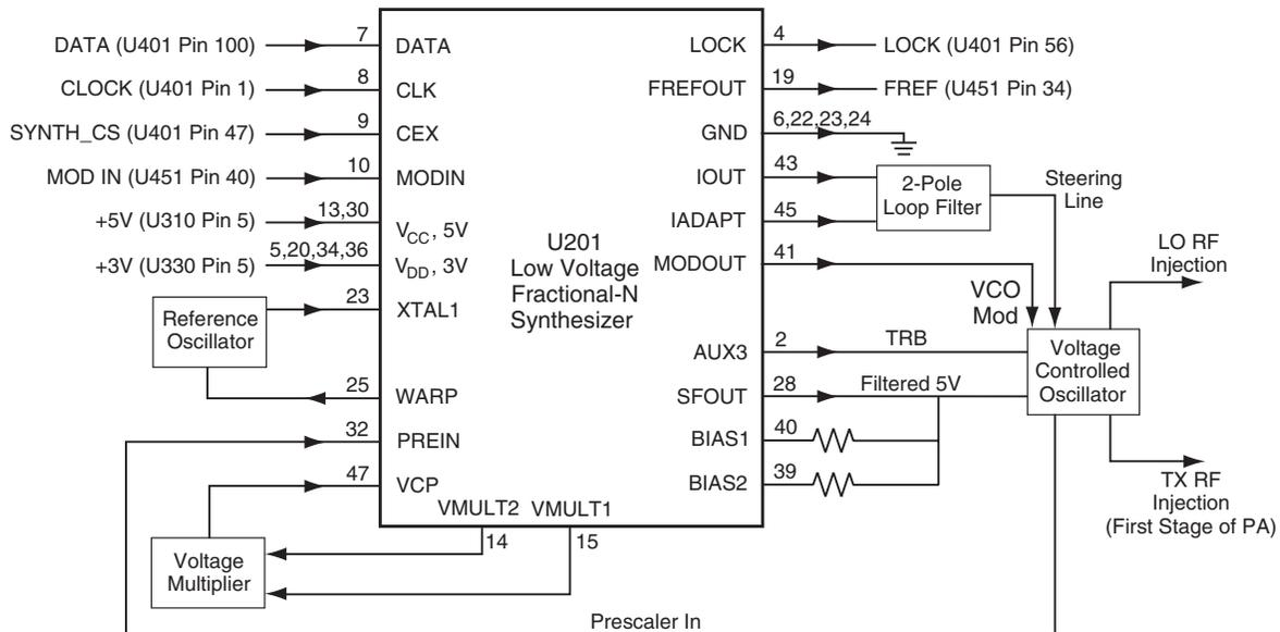
Figure 8-4. UHF Synthesizer Block Diagram
