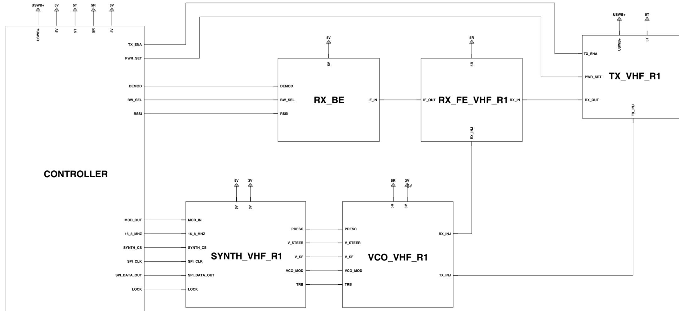
Figure 7-3. VHF (136-162 MHz) Radio Circuit Block Interconnect Diagram (8486769Z02-A)
