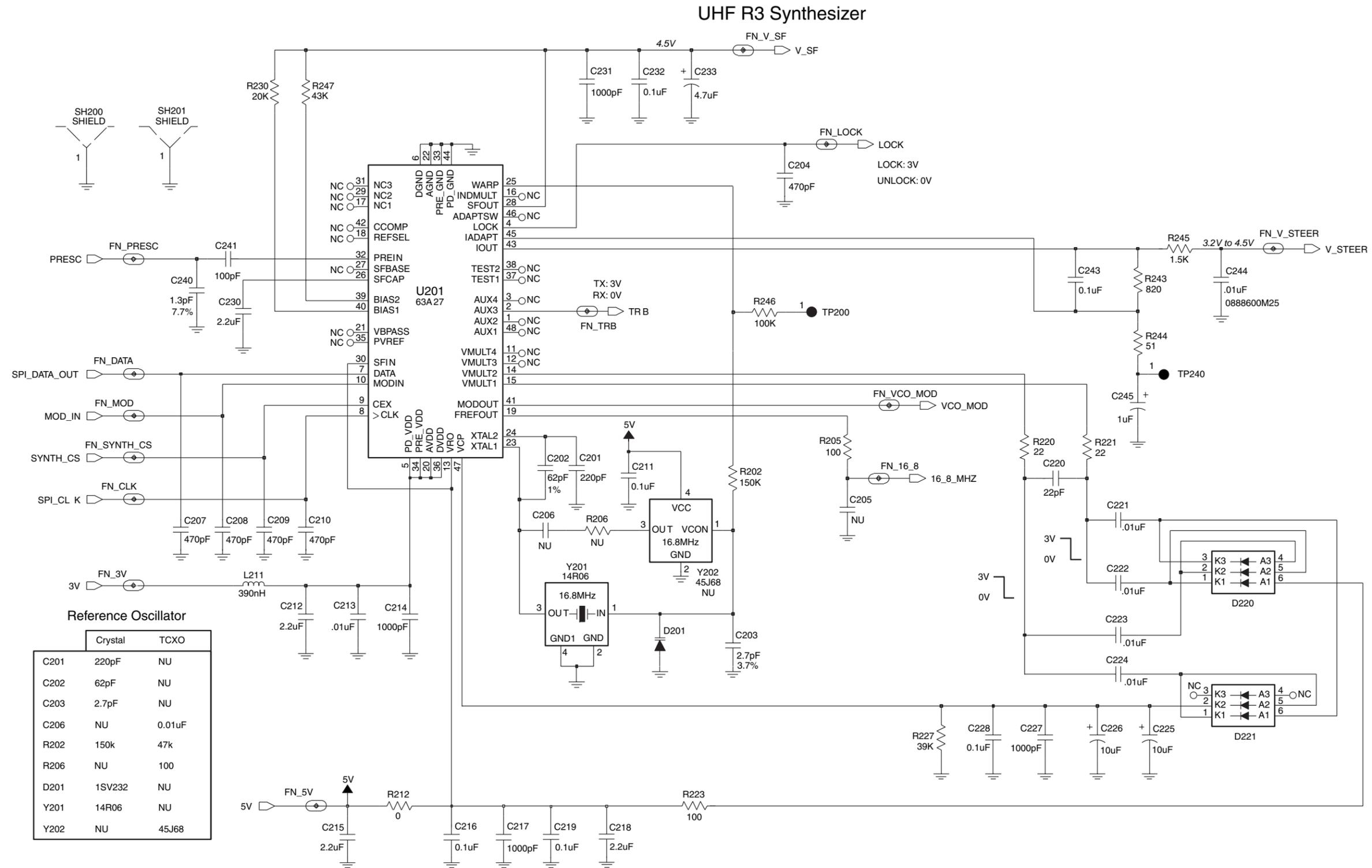
Figure 12-42. UHF (465-495 MHz) Synthesizer Schematic Diagram (8486634Z02-O)
