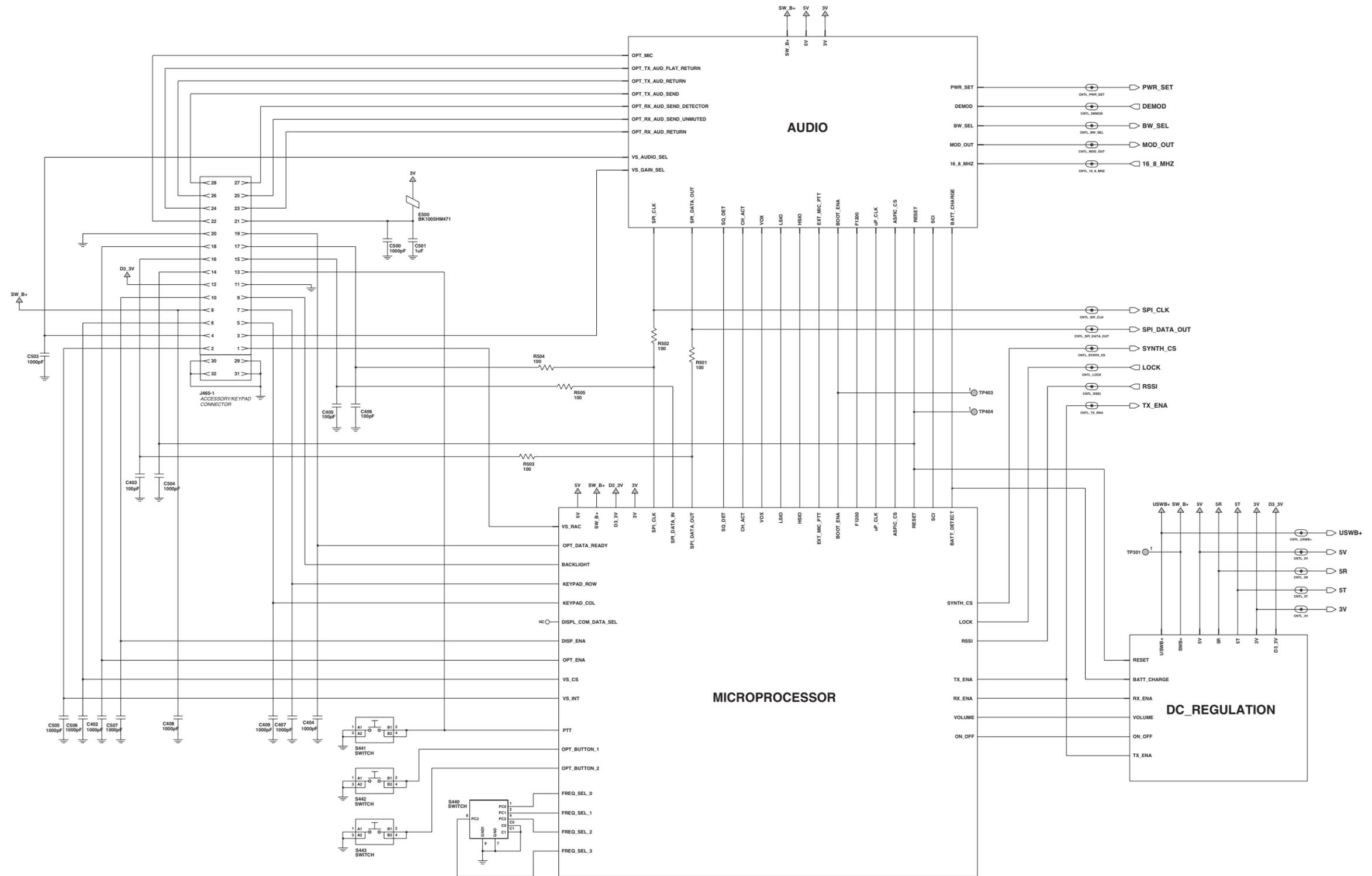
Figure 7-45. VHF (146-174 MHz) Controller Interconnect Schematic Diagram (8486342Z13-C)
